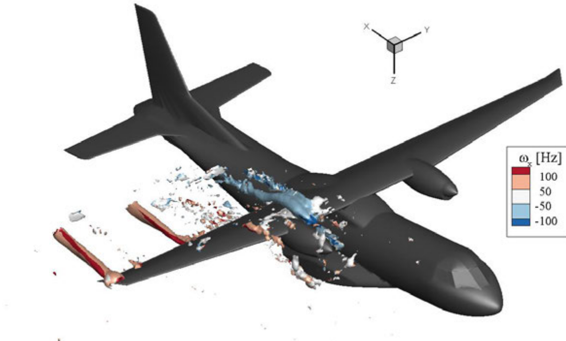
Fig. 7. Illustration of the vortical structures in the flow field. Iso-surfaces of Q-criterion ( Q = 1000 \text{ s}^{-2} ) color-coded by streamwise vorticity.
