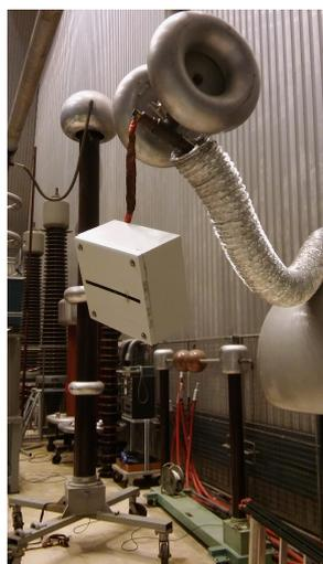
Figure C.3: Rectangular steel box under corona discharge test
