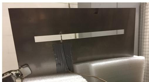
Figure C.2: Stainless steel plate of 230x125x2 mm
