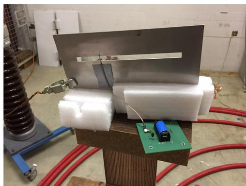
Figure C.4: Stainless steel plate under corona discharge test
