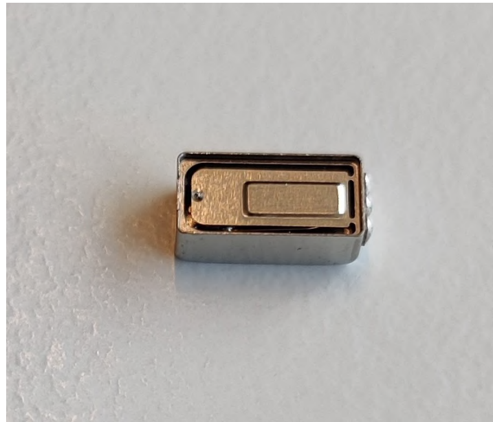
Figure 4.8: 3100 balanced armature receiver with open motor
