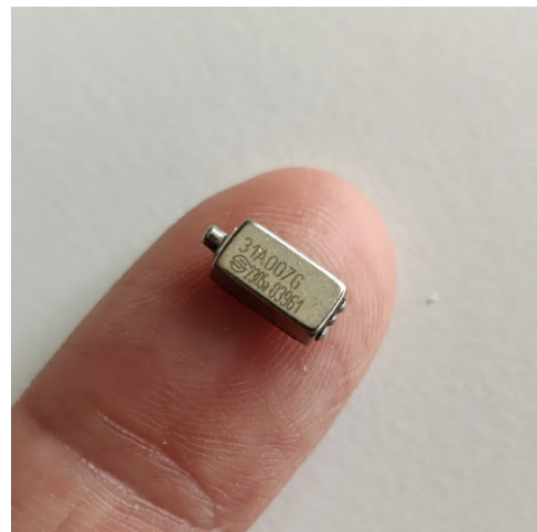
Figure 1.1: The 3100 Sonion balanced armature receiver
