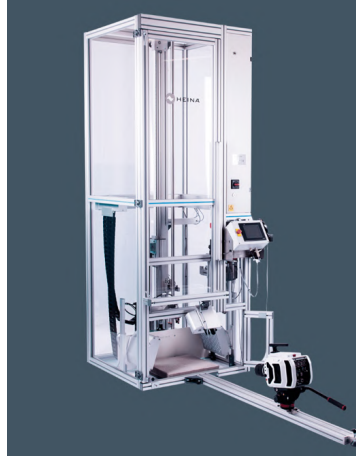
Figure 4.1: Guided Free fall (Heina DT2000) available at the research facility of Sonion Nederland B.V.
