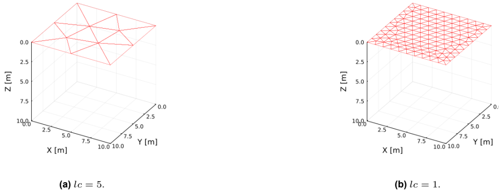
Figure 3.1: Visualisations of the mesh of the plate for two different values of lc .
