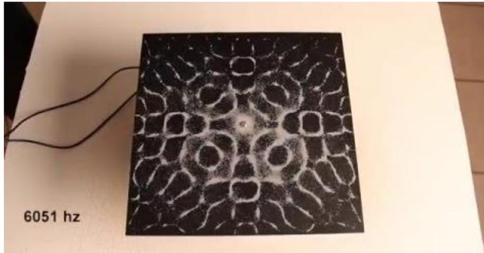
Figure 46. Example of a Chladni-figure on a rectangular plate (WEB: [geek.com/news/chladni-plate-experiment-makes-for-a-jaw-dropping-video-1558421/](http://geek.com/news/chladni-plate-experiment-makes-for-a-jaw-dropping-video-1558421/)).
