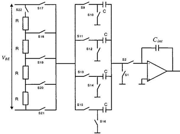
Fig. 12. Dynamic voltage divider according to [24].
