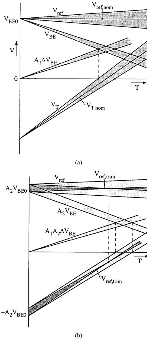
Fig. 5. Effect of spreading in  $V_{BE}$  and  $A_1 \Delta V_{BE}$  at the output voltage  $V_{ref}$  of a bandgap reference and at the output voltage  $V_T$  of a temperature sensor, before and after calibration (the curves are shown as their linear extrapolated approximations); (a) for an unscaled device ( $A_2 = 1$ ); (b) for a scaled device ( $A_2 \neq 1$ ).
