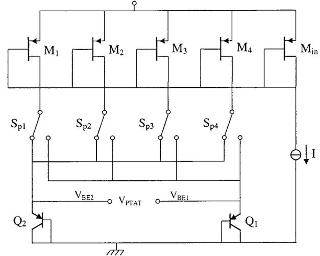
Fig. 9. Generation of  $V_{PTAT}$  using DEM, according to [20].
