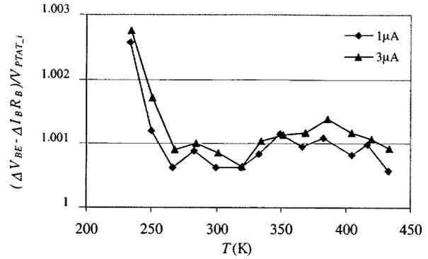
Fig. 4. Corrected  $\Delta V_{BE}(T)$  value versus the temperature.
