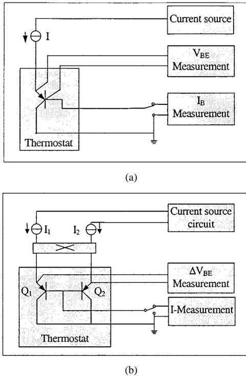
Fig. 2. Test setups to measure (a)  $V_{BE}(T)$  and (b)  $\Delta V_{BE}(T)$ .
