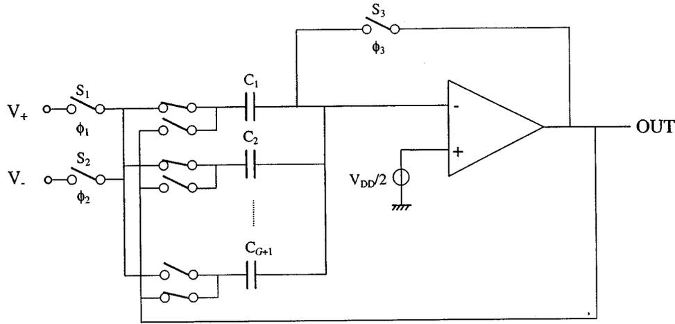
Fig. 11. DEM switched capacitor amplifier, according to [22].
