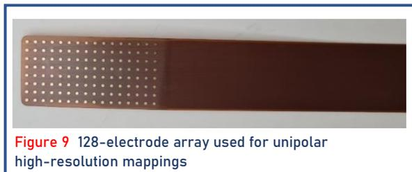
Figure 9 128-electrode array used for unipolar high-resolution mappings
