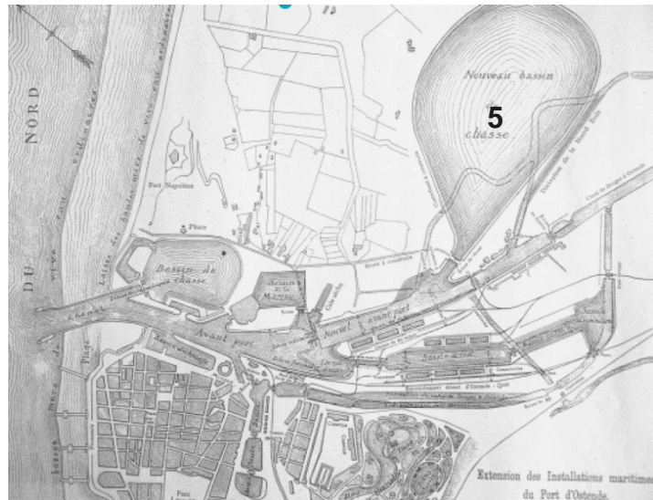
Figure 6 - Ostend flushing basins anno 1897 (Hubrechtsen, 2000)
