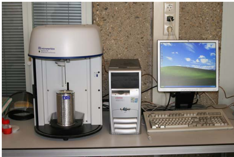
Figure 5.3 Photo of Gemini VII 2390 (nitrogen adsorption)
