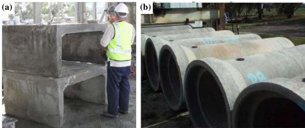
Figure 2.6 Applications of alkali activated fly ash: (a) box culverts [Lloyd and Rangan, 2010]; (b) sewer pipes [Gourley and Johnson, 2005].
