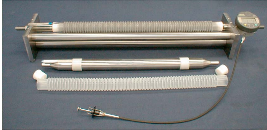
Figure 7.2 The apparatus for corrugated tube measurement for autogenous shrinkage [ASTM 1698-09, 2009]
