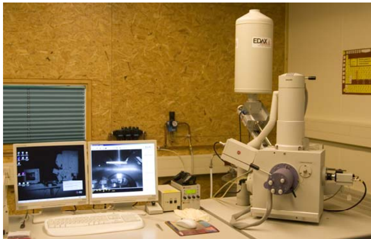
Figure 4.4 Photo of the Philips-XL30-ESEM used for ESEM observation
