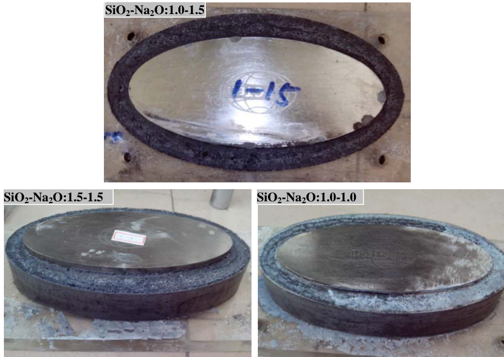
Figure 7.9 Ellipse ring test for AAFA pastes after sealed cured at 40 °C for 7 days (demolded): cracking was not observed on the surface of all AAFA pastes.
