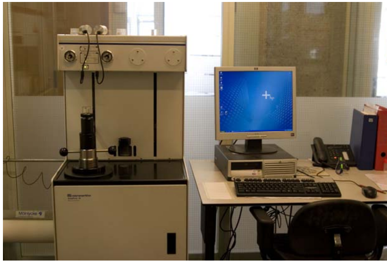
Figure 5.2 Photo of Micromeritics Poresizer 9500 (MIP)
