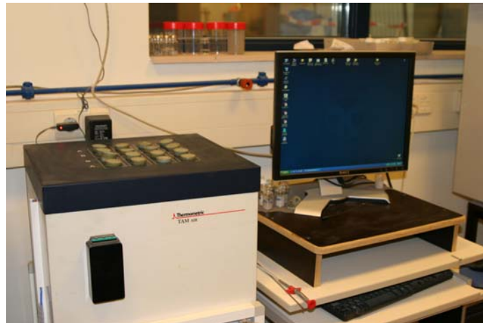
Figure 3.6 Isothermal conduction calorimeter (TAM-Air-314)
