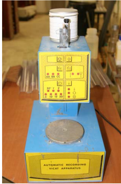
Figure 3.5 The setting time measurement by Vicat apparatus
