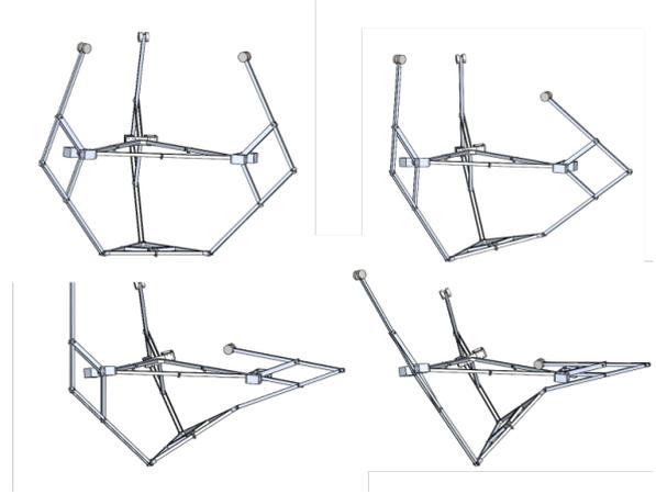
Fig. 11. CAD model of the current manipulator transitioning from translation mode to mixed freedom mode. As the center moves away from the center's vertical axis the tilt angle increases.
