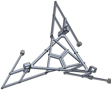
Fig. 26. The force balanced spherical parallel 3-RRR operation mode
