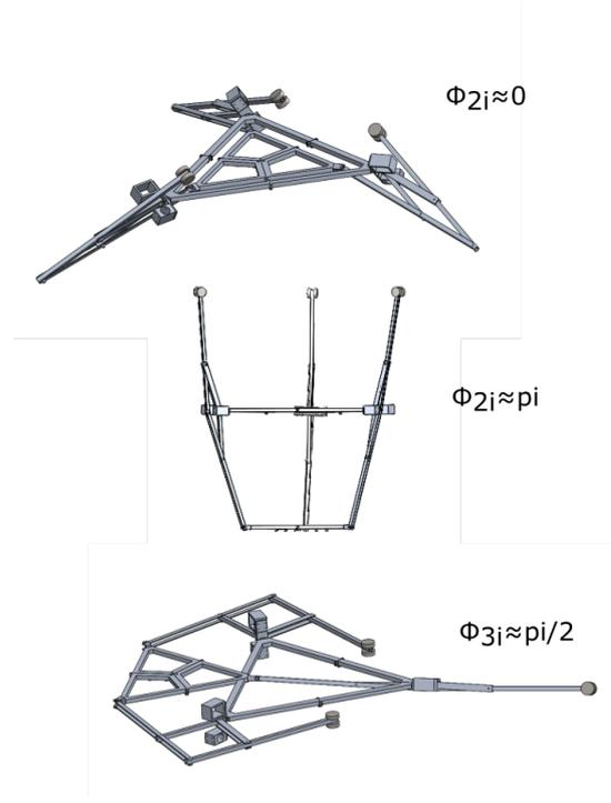
Fig. 9. CAD model of the current manipulator in its singular conditions. The first figure corresponds to the situation when the legs fold in. The second figure corresponds to the case when the legs are completely stretched out. The third figure corresponds to the situation when the legs are sideways. These in turn define the boundary of the workspace.
