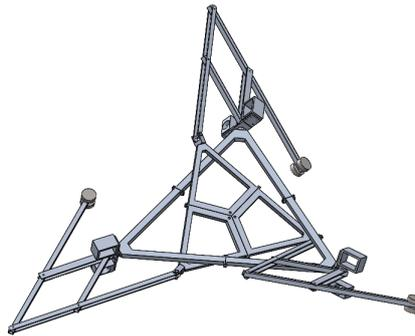
Figure 4.2: The force-balanced spherical parallel 3-RRR operation mode
