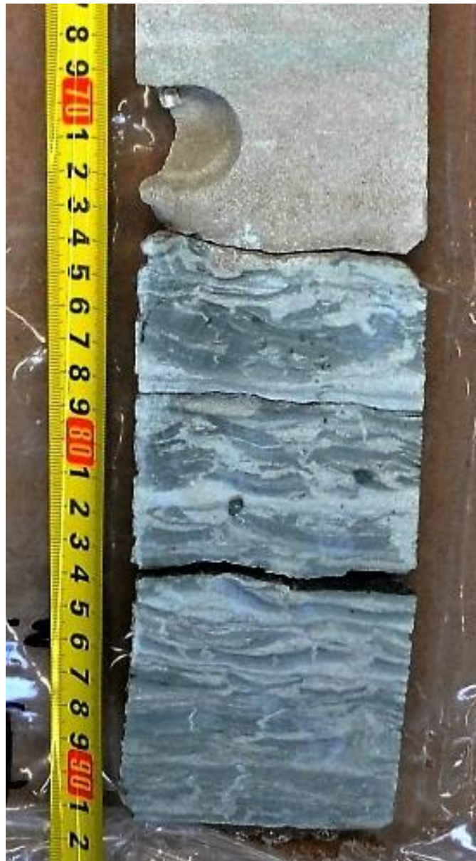
Figure 14. Clay and sand layers with desiccation or syneresis cracks. P11-02, 2376 m.
