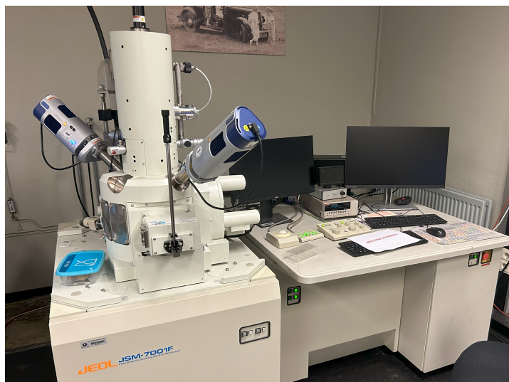
Figure 4.6: The SEM-EDS used for point analysis and scanning tiles is this JEOL 7001F.
