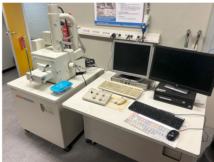
Figure 4.5: The SEM-EDS used for point analysis is this JEOL 5900LV.
