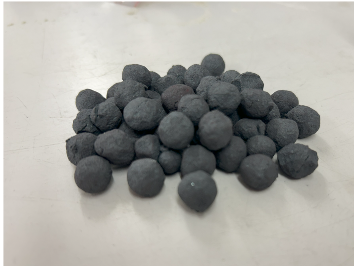
Figure 3.3: Fired pellets with IOA ores, produced for this research.
