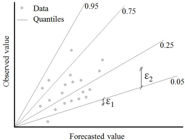
**Figure 1.** Quantile regression example scheme considering different quantiles.
