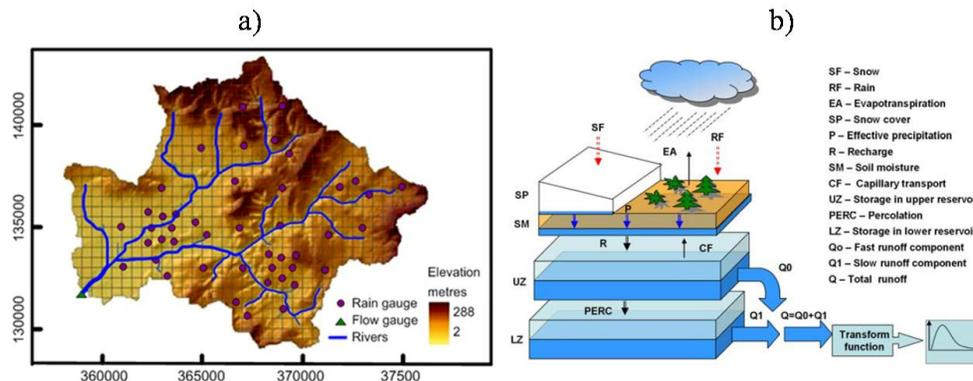
**Figure 3.** (a) The Brue catchment showing dense rain gauges network and its river gauging station, Lovington, where the discharge is measured, and (b) schematic representation of HBV-96 model (Lindström et al., 1997) with routine for snow (upper), soil (middle), and response (bottom) (Shrestha and Solomatine, 2008).
