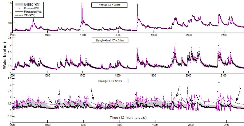
**Figure 14.** Comparison of prediction limits for 90% confidence level during validation (1 April 2012–7 March 2013): **(a)** Yeaton, lead time = 3 h, **(b)** Llanyblodwel, lead time = 6 h, **(c)** Llanerfyl, lead time = 12 h.
