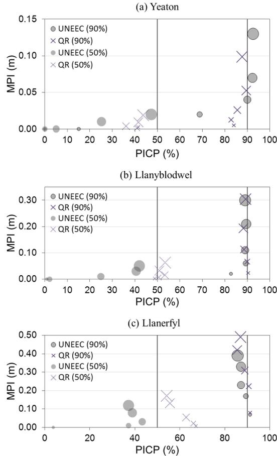
**Figure 13.** Comparison of UNEEC and QR based on both MPI and PICIP during validation period (7 March 2010 20:00–7 March 2013 08:00) for 90% confidence level (the size of the marker represents the lead time, i.e. bigger the marker, longer the lead time).
