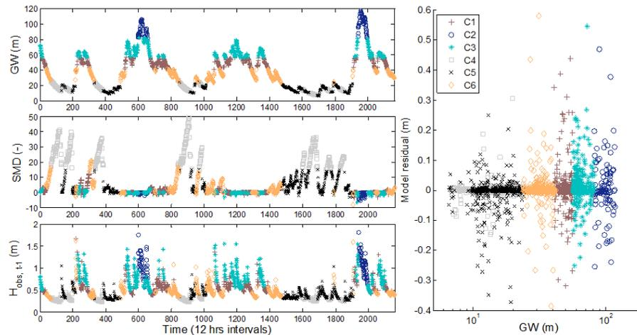
**Figure 5.** Fuzzy clustering of:  $GW$  (left, top) and its relation with the model residuals (right),  $SMD$  (left, middle) and  $H_{obs,t-12}$ , (left, bottom) for calibration period (7 March 2007 08:00–7 March 2010 08:00) – Llanyblodwel, lead time = 6 h.
