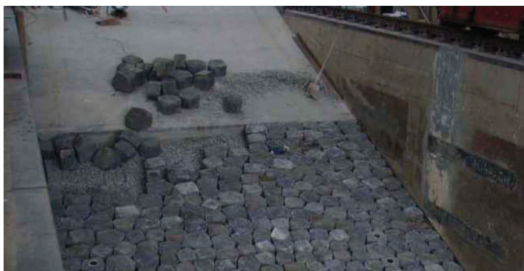
Figure 6–28 Picture of revetment construction in the Delta flume (source: Van Steeg & Klein Breteler, 2009)
