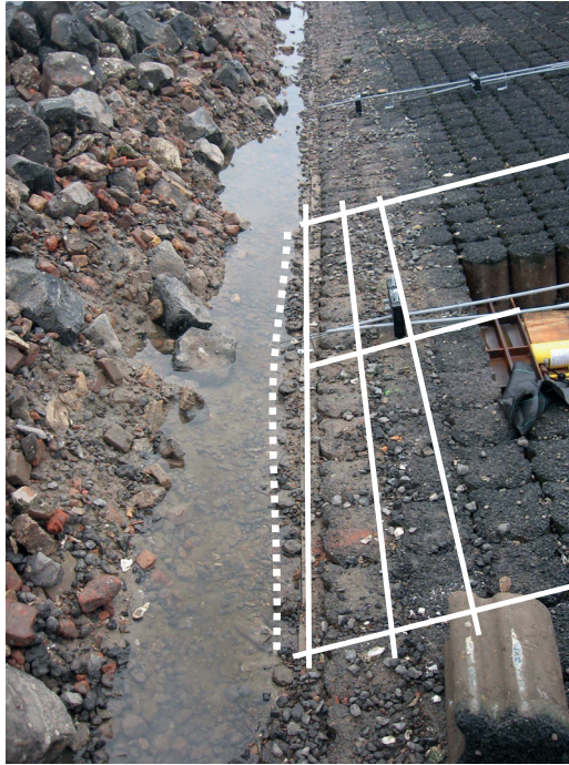
Figure H-4 Observed toe permanent deformation on location C
