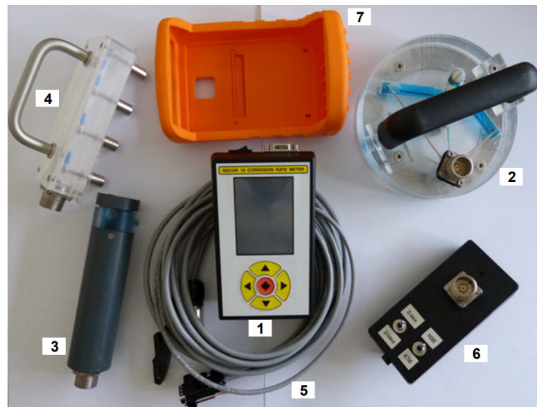
Figure 2.6: The Gecor-10 measurement device with all its components: 1) Gecor-10 main unit, 2) confinement sensor, 3) Potential sensor, 4) 4-tip resistivity sensor, 5) cables, 6) calibration box, and 7) protective housing. [44]
