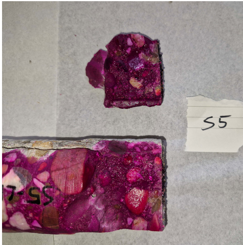
Figure F.5: Carbonation of core S5-CL1
