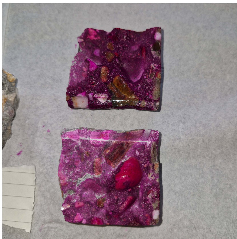
Figure F.8: Carbonation of core L17-CL1
