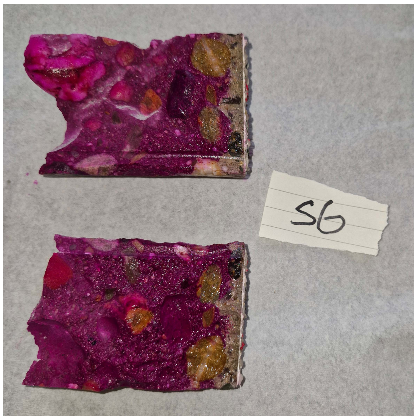
Figure F.10: Carbonation of core S6-CL1
