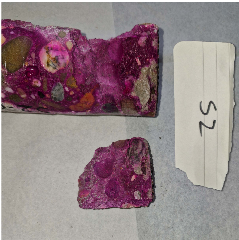
Figure F.3: Carbonation of core S2-CL1
