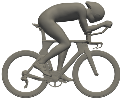
Figure 3.3: CAD of the Symmetric GCM on the bike
