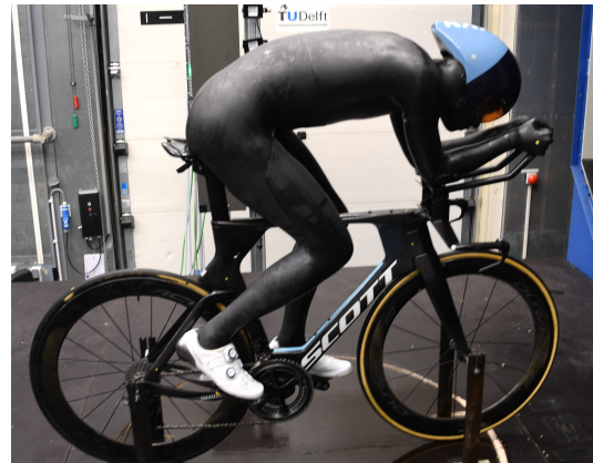
Figure 3.4: Printed symmetric GCM placed on the bike
