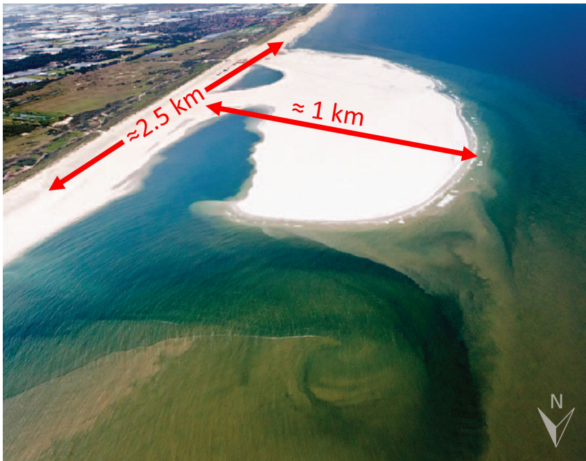
Figure 4.1: Aerial photograph of the Sand Motor after completion (September 2011). Note the clouds of fine-grained material moving to the North. Picture courtesy of Rijkswaterstaat / Joop van Houdt
