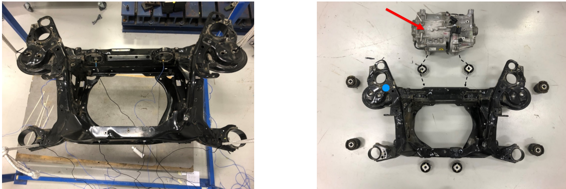
Figure 1: On the left, a picture of the SEMM measurement set-up. On the right, an overview of the FBS case. The red arrow indicates the force excitation, the blue circle the location of the validation sensor.
