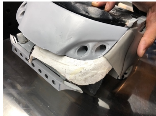
Figure 43: Support structure with bonnet
