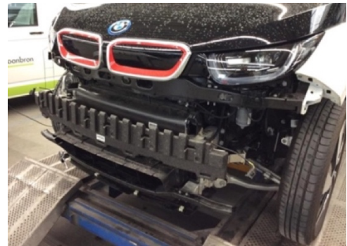
Figure 17: Photograph of BMW i3 with removed front bumper
