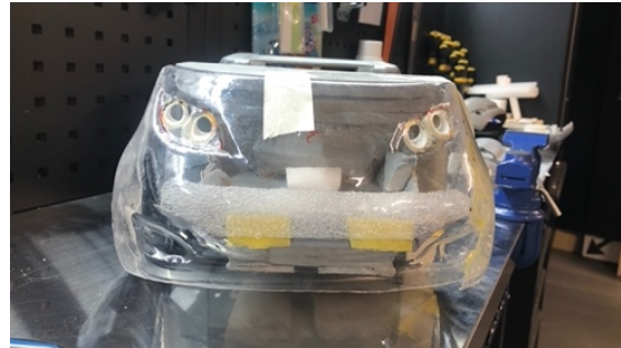
Figure 46: Existing front clip with extended bumper beam and energy absorber
