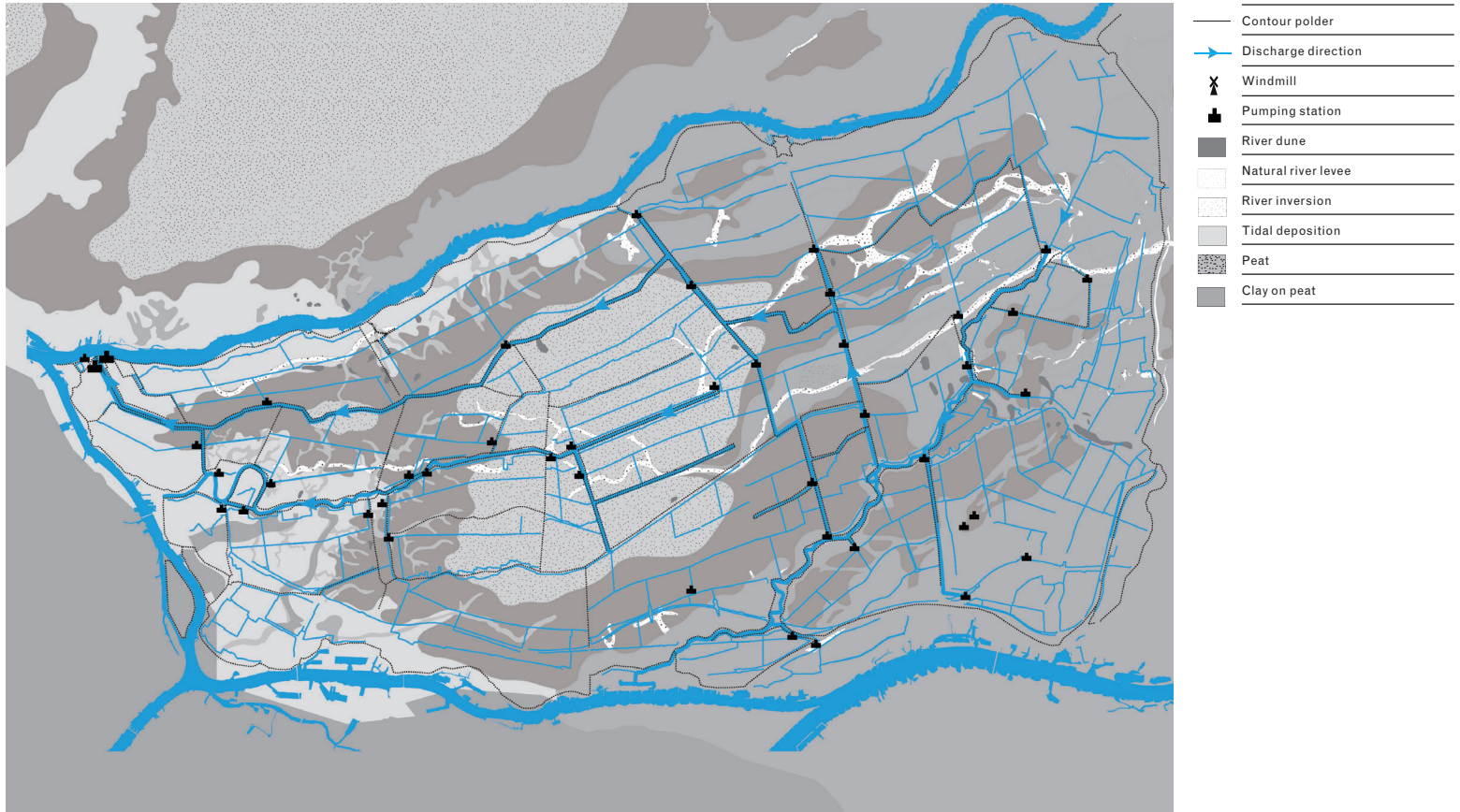
Water pattern and discharge direction of polder complex Alblasterwaard projected on the natural landscape
