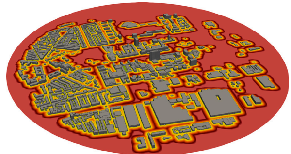
Fig. 9. SDF generated for the Delft University of Technology central campus with a background grid size of 2 Billion grid points and 25 Million triangulation faces for the underlying geometry. Only a section of the grid is shown in the figure.
