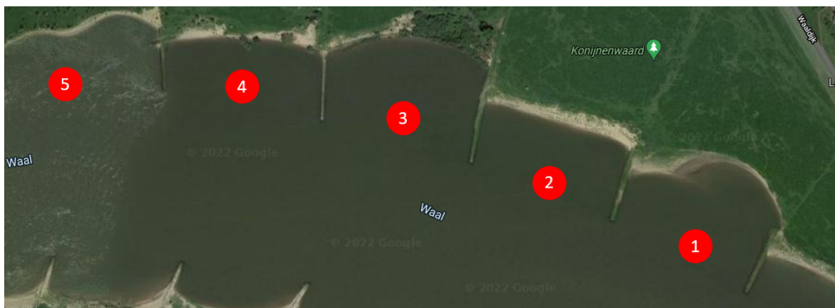
Figure A.2: Groyne field pilot locations near Haalderen. Groyne field one will be used as a reference groyne field while groyne fields two to five will be used for the actual nourishments.
