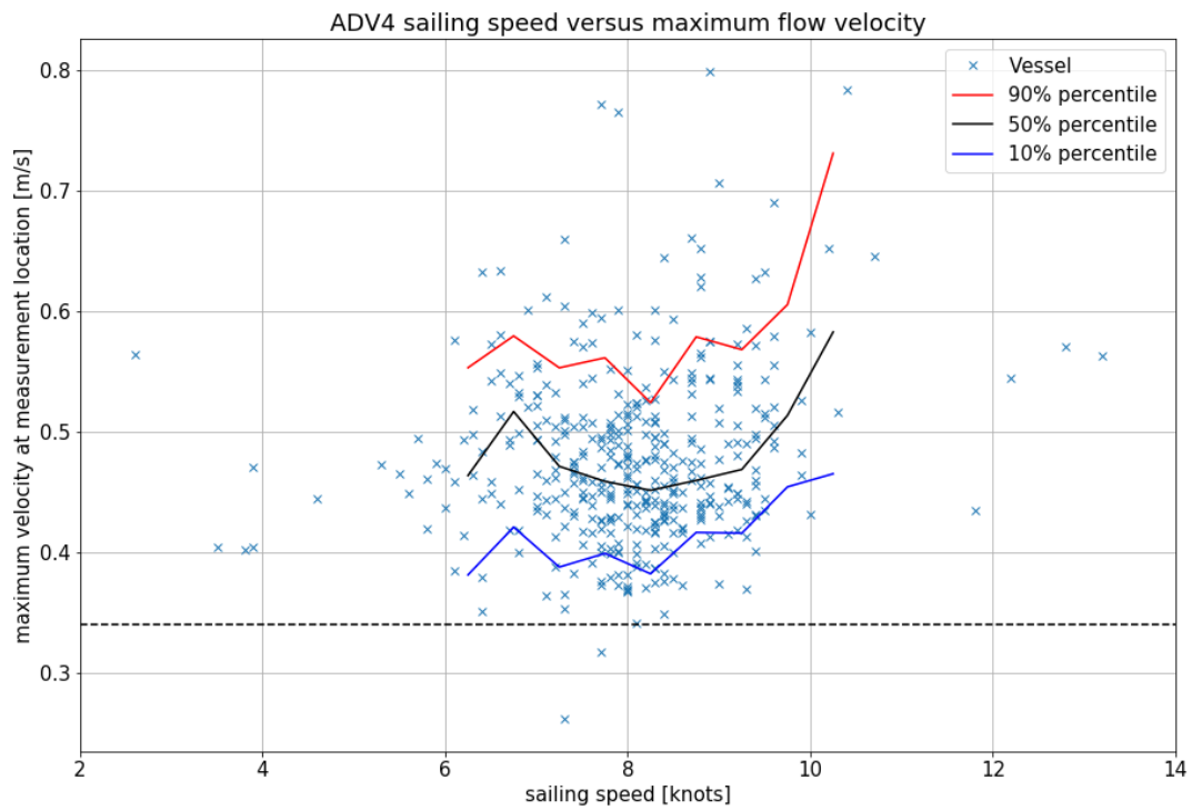
Figure E.34: ADV4 sailing speed versus maximum flow velocity at measurement location
