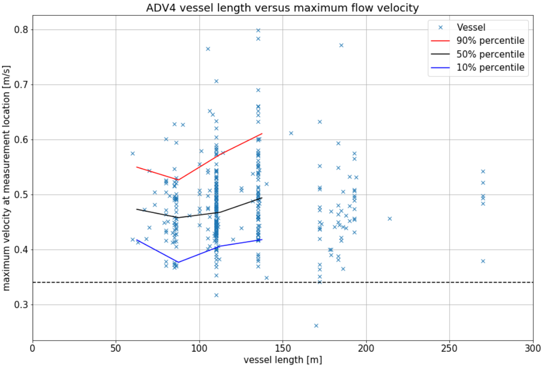
Figure E.37: ADV4 vessel length versus maximum flow velocity at measurement location
