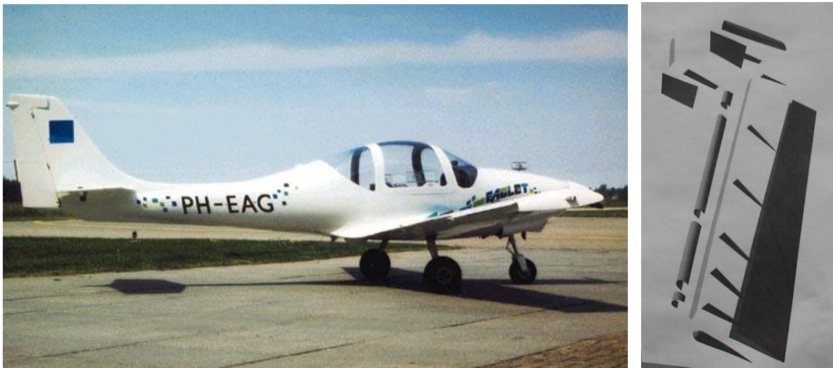
Figure 5.11 The two seater “eaglet” (left) and an exploded view of its rudder with its components (right).
