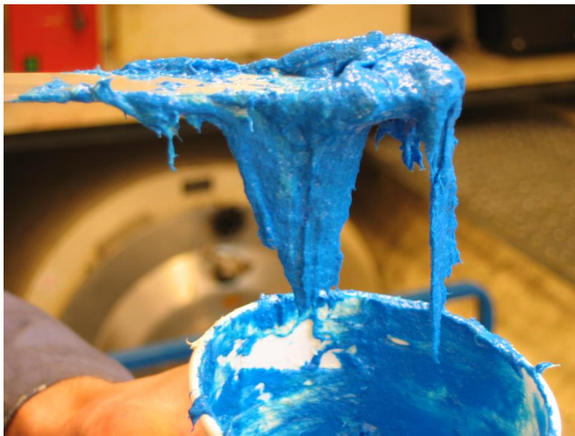
Figure 4.15 Rubber compound with 1% of Twaron pulp.
