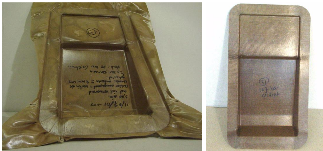
Figure 1.4 Product development of a rubber formed part produced at the Structures and Material Laboratory.
