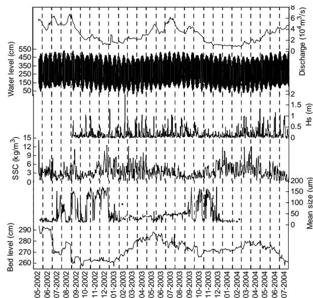
Figure 1: Time series of river discharge, water level, significant wave height, SSC, mean size and bed level.
