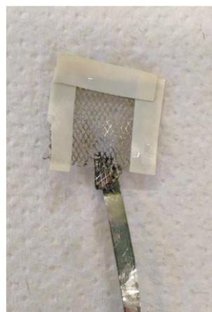
Figure 7: Electrotaped anode before electroplating. This is done to ensure metal-metal contact for welding is possible with the bipolar plate and the anode. The area for electroplating is 1x1 cm.
