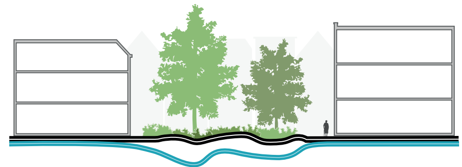
Figure 11.14. Schematic: effect of vegetation on the groundwater level
