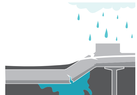
Figure 3.11. Subsidence-damaged sewers (based on image shown during interview with A. Fijan, personal communication, may 2015)
