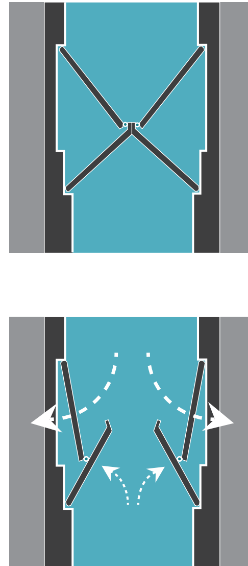
Figure 3.5. Dark Sluice schematic (Denslagen, 2001)
