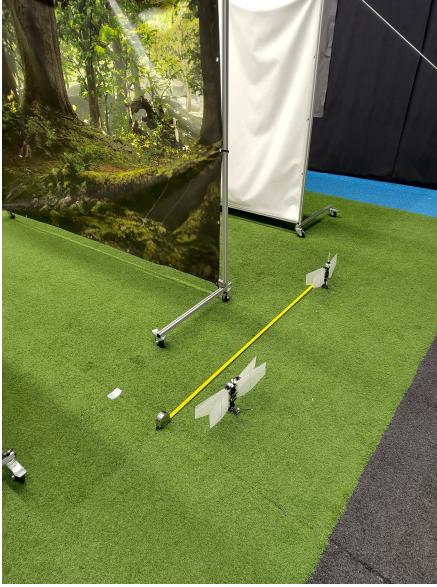
Figure 9: Photo of the initial test setup in the CyberZoo. The Flappers are spaced 1.50 m apart at first and facing towards aisles that are supposed to mimic crop rows in a greenhouse.
