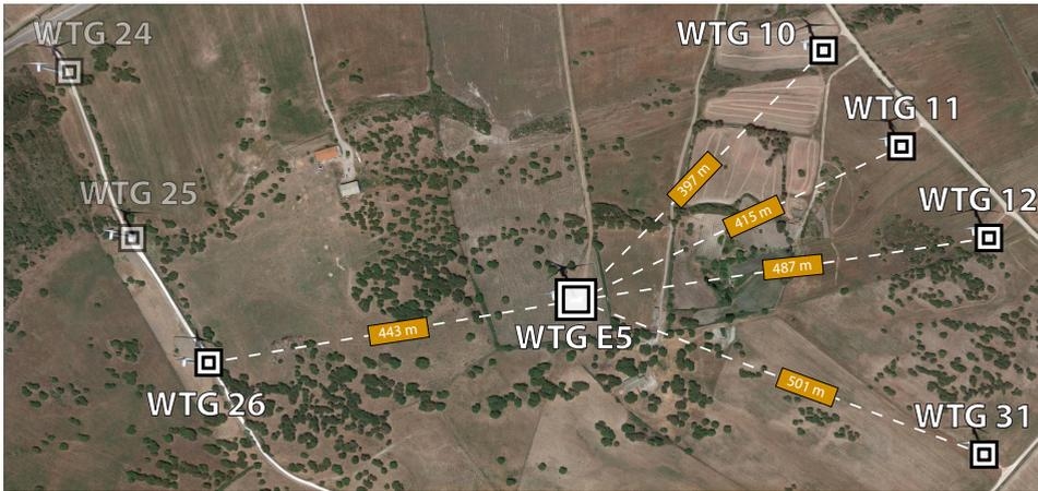
Figure 2.1: Positions of the wind turbines used in the wake steering campaign. Turbines WTG 26 and E5 are operated at a yaw misalignment to steer the wakes away from downstream turbines WTG E5, 10, 11, 12 and 31. WTG 25 is used for normalization. WTG E5 is a GE 1.5sle turbine and all others are GE 1.5s turbines. Imagery ©2020 Google, Imagery ©2020 CNES / Airbus, Maxar Technologies, Map data ©2020.
