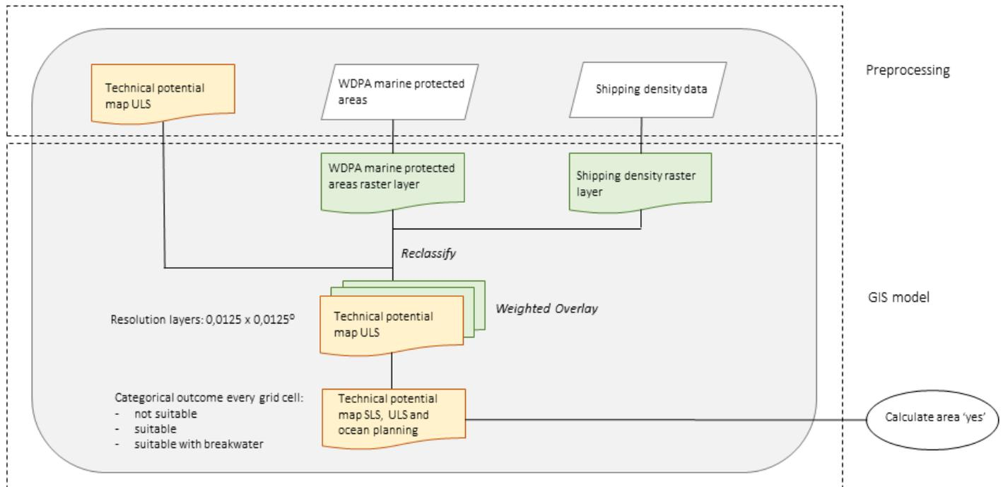
Figure 3.3: Workflow diagram technical potential map ocean planning
