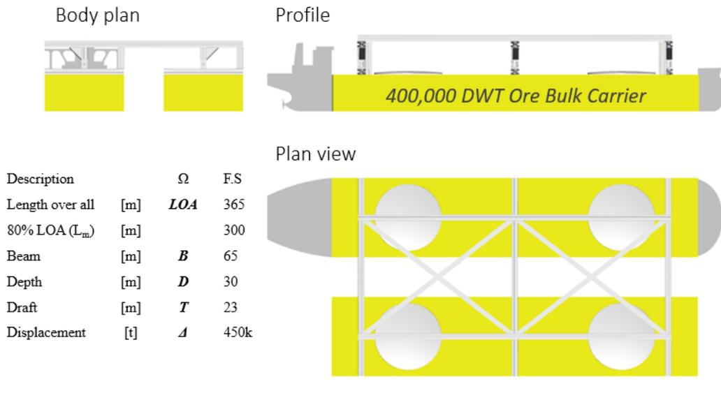
Figure 2.4: Proposed design of floating breakwater, as presented in G. Wang et al. (2023)
