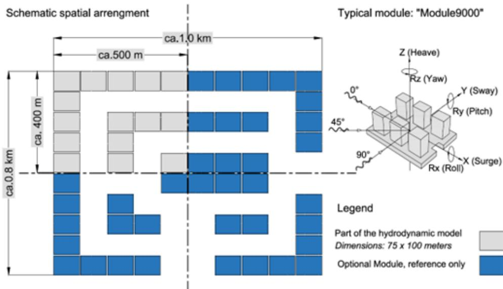
Figure 2.3: Spatial arrangement of MFS “twin-hull” modules, as presented in G. Wang, Drimer, and Goldfeld (2020)
