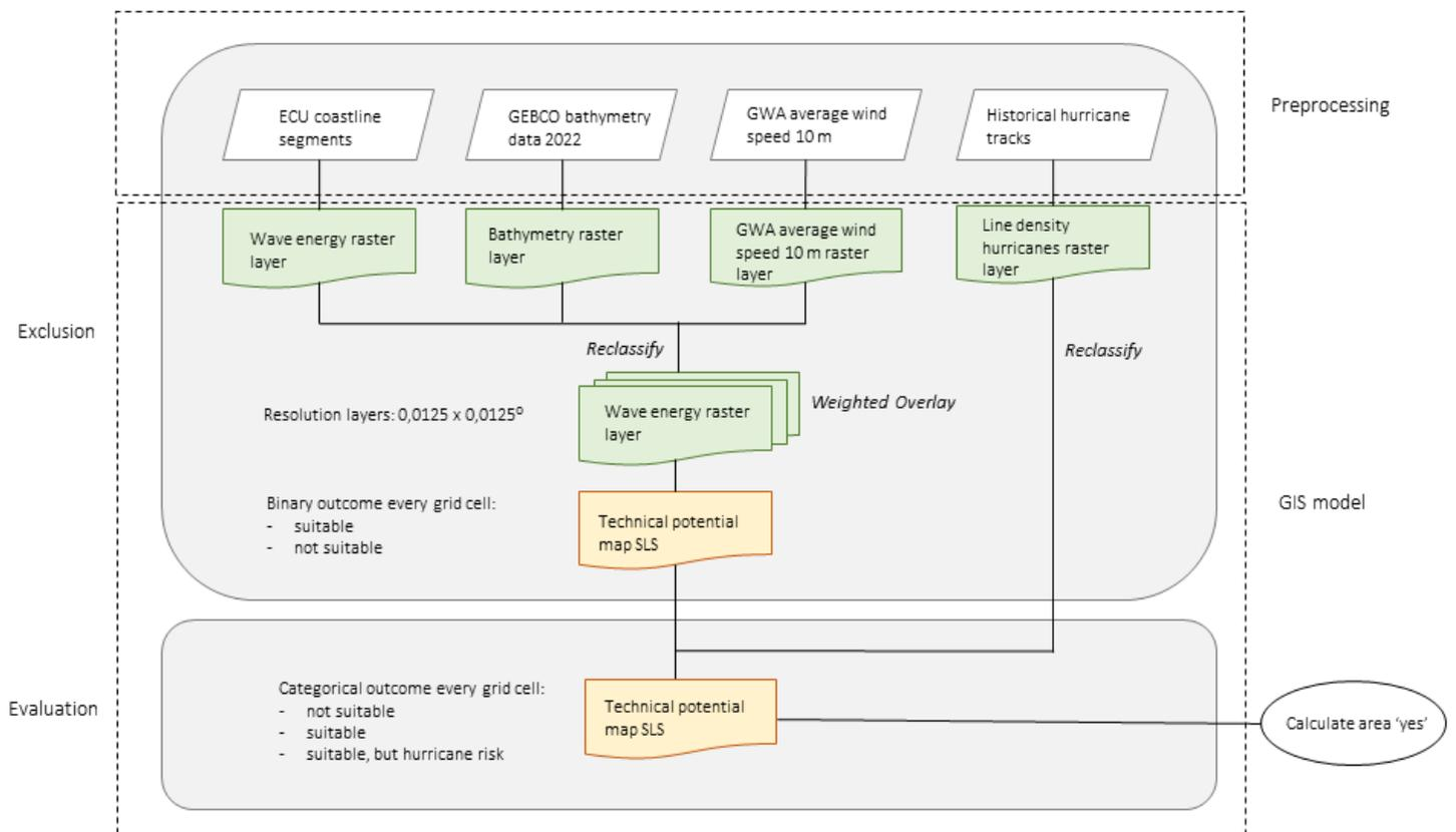
Figure 3.1: Workflow diagram technical potential map Service Limit State (SLS)
