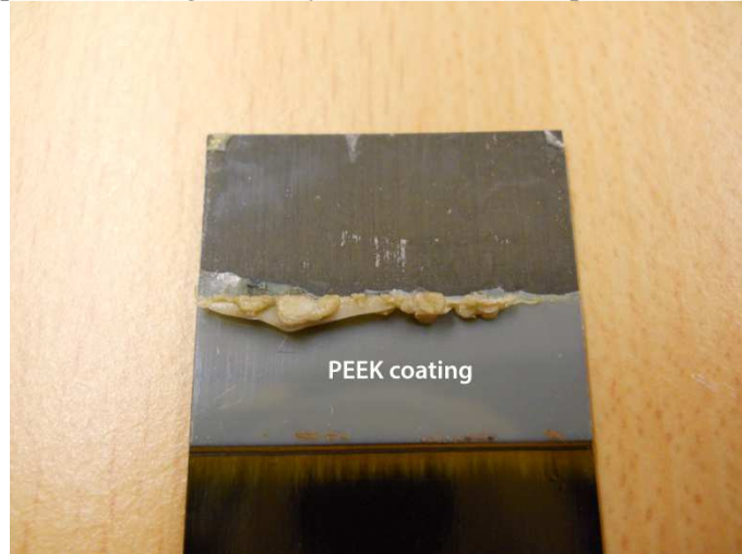
Figure 5: Fracture surface of the CF/epoxy adherend after indirect welding on a co-cured PEEK layer under short-welding-time conditions (460 ms). Only adhesive failure can be observed here.
