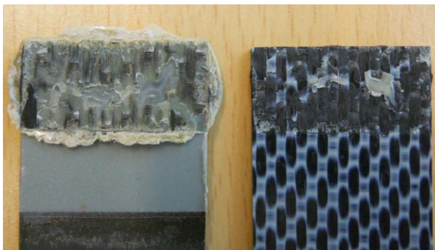
Figure 6. Fracture surfaces of a CF/PEEK to CF/epoxy indirect weld with improved adhesion between the CF/epoxy and the PEEK coating layer co-cured to it. Failure mostly occurs in the CF/PEEK composite substrate (right).
