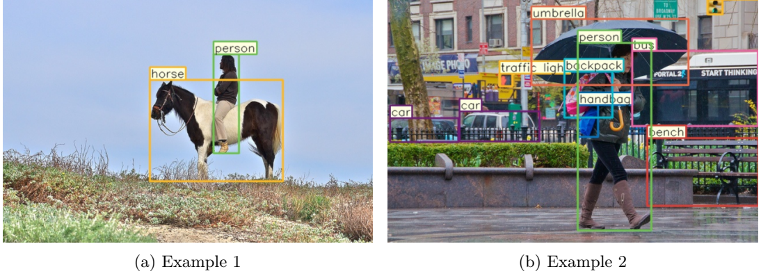
Figure 2.2: Output of an object detection network for two images from the MS COCO dataset. Detected objects are classified and located with a bounding box.
