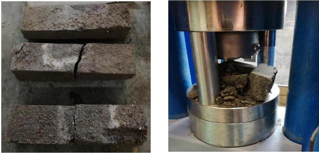
Figure 55: Mortar prisms containing thermally treated CEM I before and after testing. The prisms crumbled or parts broke off and no measurable strength results were obtained.
