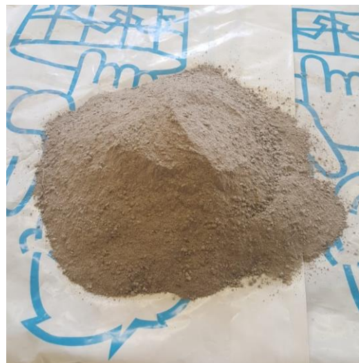
Figure 31: Smart Crusher material of the 0 - 4 mm fraction before sieving.
