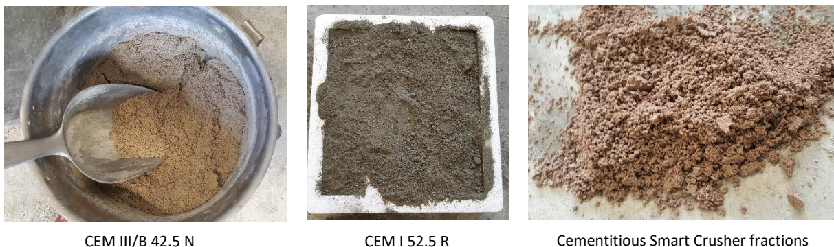
Figure 53: Mortar mixtures containing thermally treated cementitious binder showing the rather dry consistency of the mixtures.
