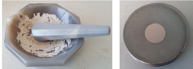
Figure 36: Sample preparation for XRD analysis. Grinding the material into a fine powder before compressing the powder in an aluminium holder, which can be placed in the diffractometer.
