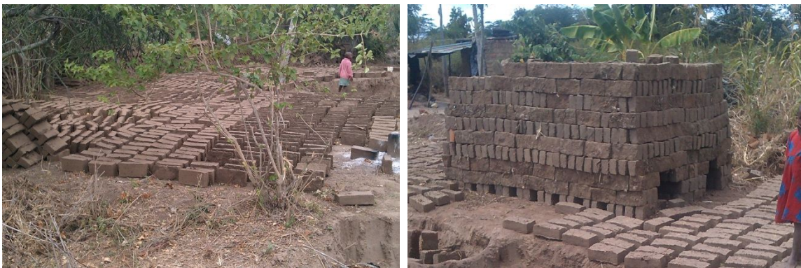
Figure A.82 Brick making site. Bricks drying (left); preparation for burning the brick (right)
