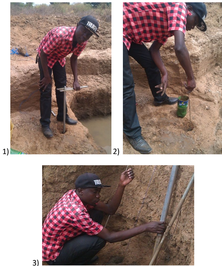
Figure C.2 Execution steps of the Auger hole method
