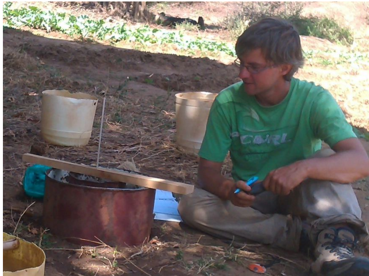
Figure C.7 Execution of the double ring infiltration test
