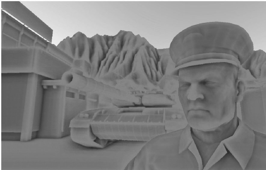
Figure 2.3: SSAO as originally introduced by Cytek. Note how even flat surfaces without any occlusion appear to be 50 % occluded (grey). [2]
