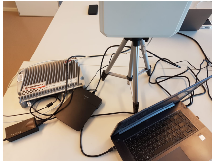
Figure 3.5: Picture of the RFID reader connected to a laptop running the reader interface
