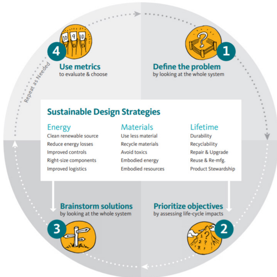
Figure 11: Whole Systems and Lifecycle Thinking for sustainable design. Source: Autodesk Sustainability workshop.
