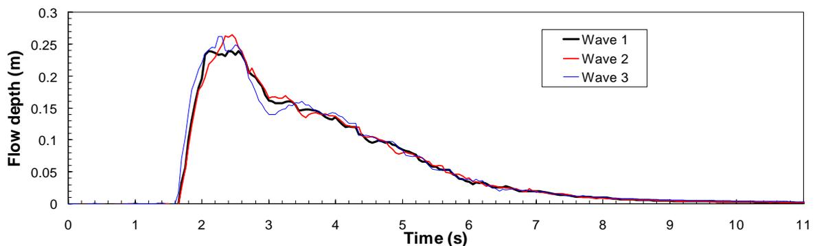
Figure 5. Record of flow depth with floating device for 3 overtopping waves of  $3 \text{ m}^3/\text{m}$
