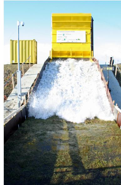
Figure 1. Principle of Wave Overtopping Simulator
