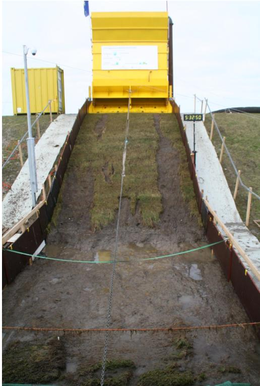
Figure 17. Afsluitdijk. Toe with grass on clay.
