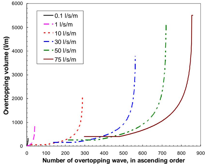
Figure 4. Distribution of overtopping volumes of waves for sea dikes and various mean overtopping discharges, as simulated by the Wave Overtopping Simulator.
