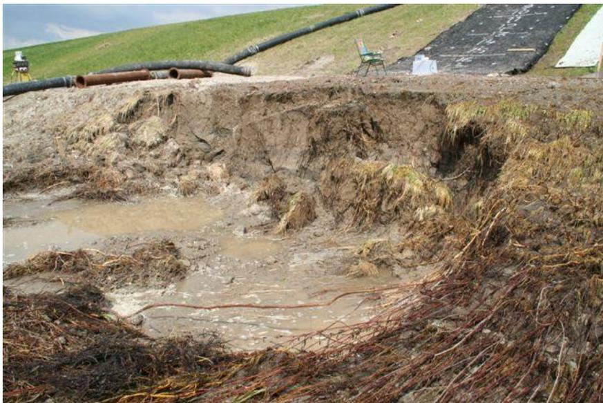
Figure 16. Final result Kattendijke, Zeeland; open asphalt concrete.
