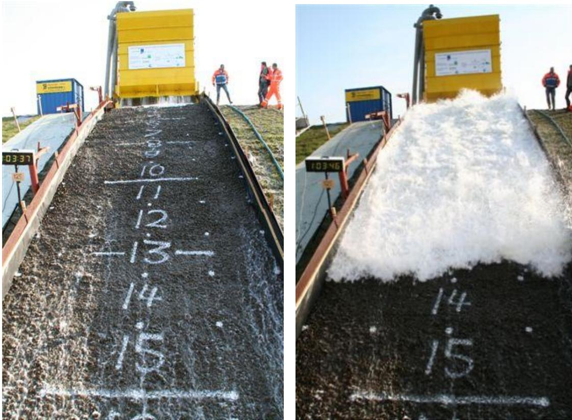
Figure 15. Kattendijke, Zeeland. Final test on elastocoast.
