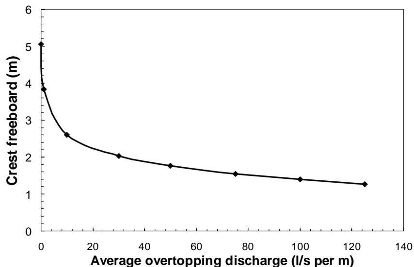
Figure 21. Relationship between overtopping discharge and required crest freeboard ( $H_s=2$  m;  $s_{op}=0.04$  and  $\cot\alpha=4$ )
