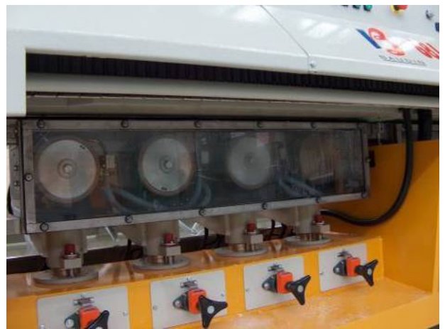
Figure 26, Clip-Edge cutting machine. 6 individual cutting blades produce the odd-shaped groove.
