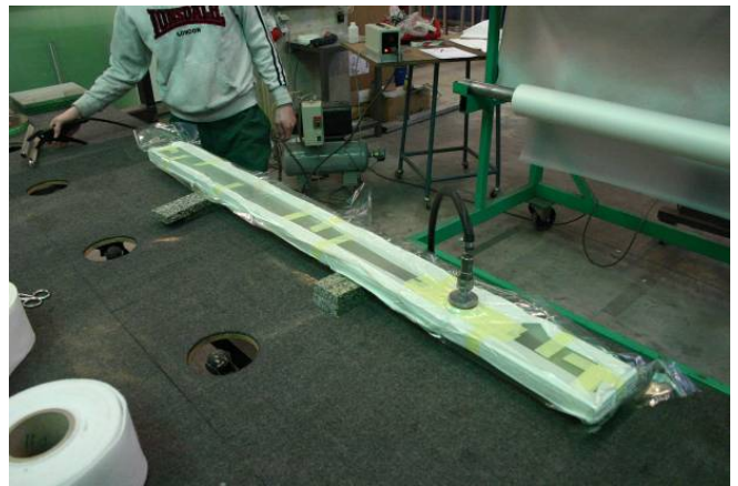
Figure 31, Laminating process with SGP film, from right to left, top to bottom:
