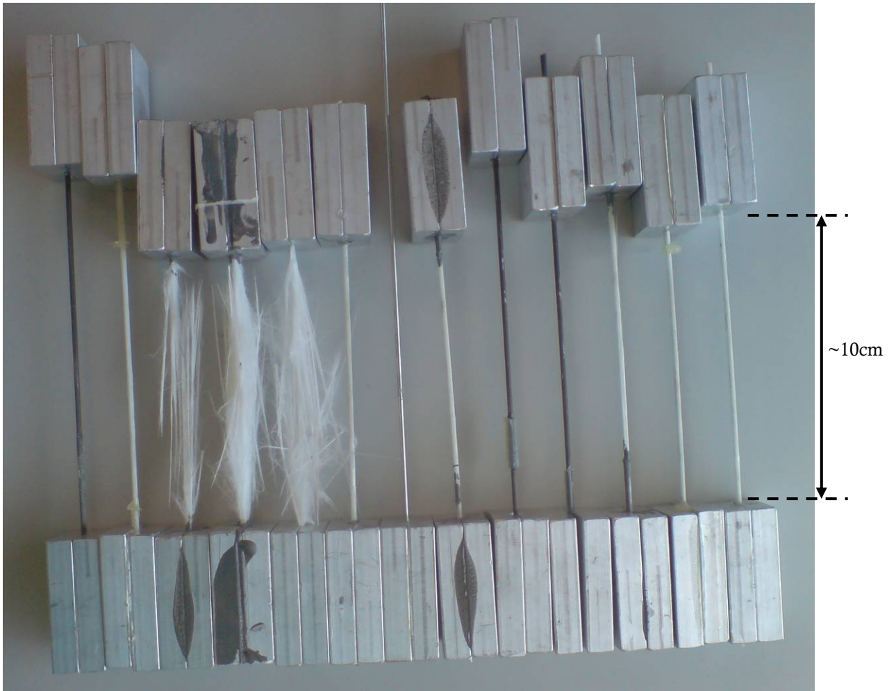
Figure 92, 13 tested specimens after the tests. Specimens consist of \varnothing 2\text{mm} bars adhesively bonded in aluminum blocks with different adhesive thicknesses.
