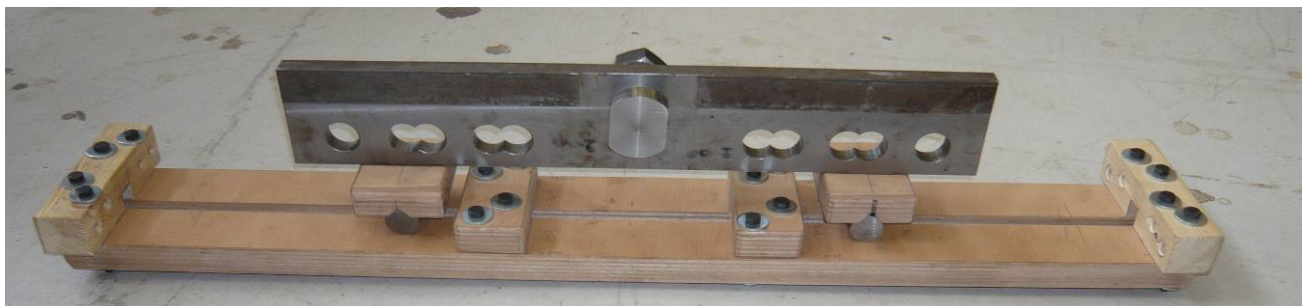
Figure 125, Altered upper support flange.
