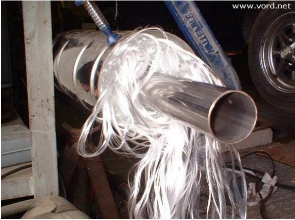
Figure 74, E-Glass fiber, here in use as sound buffer in an exhaust pipe of a car. [28]
