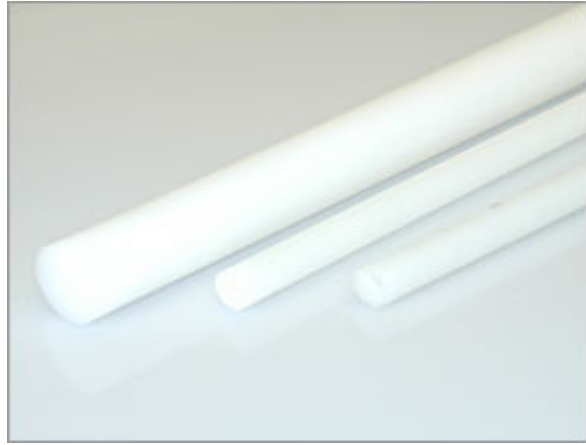
Figure 73, Pultruded glass fiber rods. [28]
