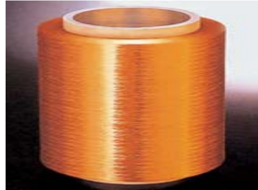
Figure 58, Zylon on Spool [28]
