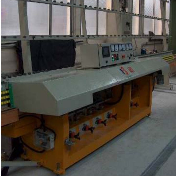
Figure 26, Clip-Edge cutting machine. 6 individual cutting blades produce the odd-shaped groove.
