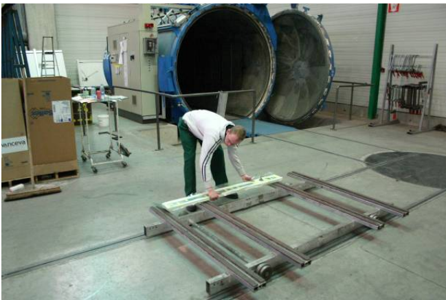
Figure 31, Laminating process with SGP film, from right to left, top to bottom:
