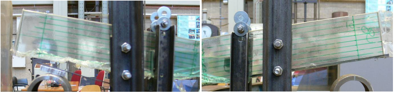
Figure 155, Left and right end of specimen 90-01 after collapse.
