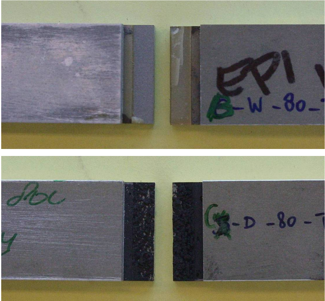
Figure 33 a+b, a (above): 100% adhesive failure where adhesive is stuck on 1 substrate. b (below): 100% cohesive failure, where adhesive is stuck on both substrates.[18]
