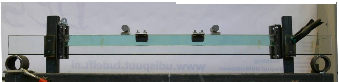
Figure 132, Girder in setup, isolated from the bench press.
