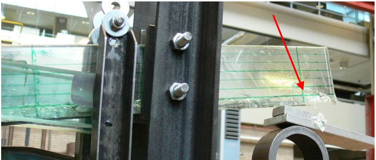
Figure 140, Specimen 70-03 after the test with the broken reinforcement (encircled above). The end of the reinforcement is denoted by the arrow in the bottom picture.
