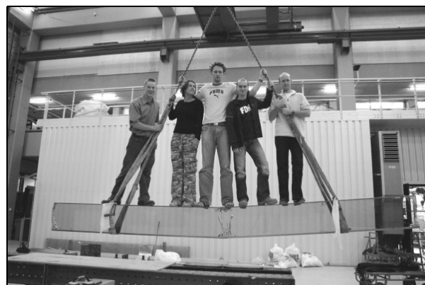
Figure 50, Proof of residual load bearing strength of stainless steel reinforced glass beam. [12]
