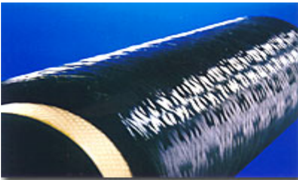
Figure 69, Carbon fiber yarn on spool [28]
