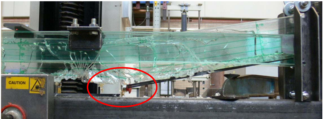
Figure 141, Close-up of specimen 70-03 200mm left of the center of the girder. The cracks run up far in to the top of the girder under the support (encircled in red).
