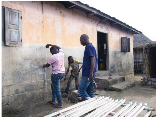
(c) Taking 2010 flood mark measurements (own work)
