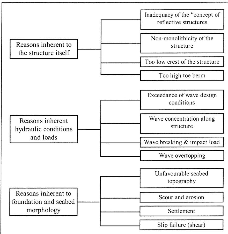
Figure 7-1 Reasons of failure of vertical breakwaters [Oumeraci 1994]
