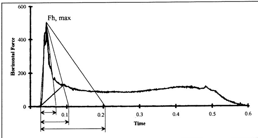
Figure 5-22 Schematising impact duration, method 1
