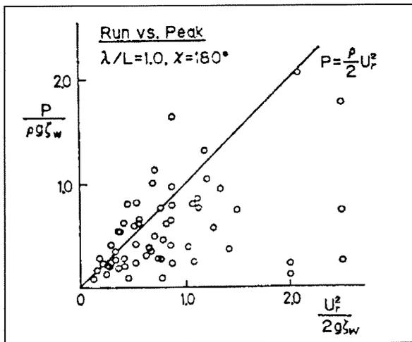
**Figure 5-5 Comparison of measured and calculated impact pressure [Watanabe 1987]**
