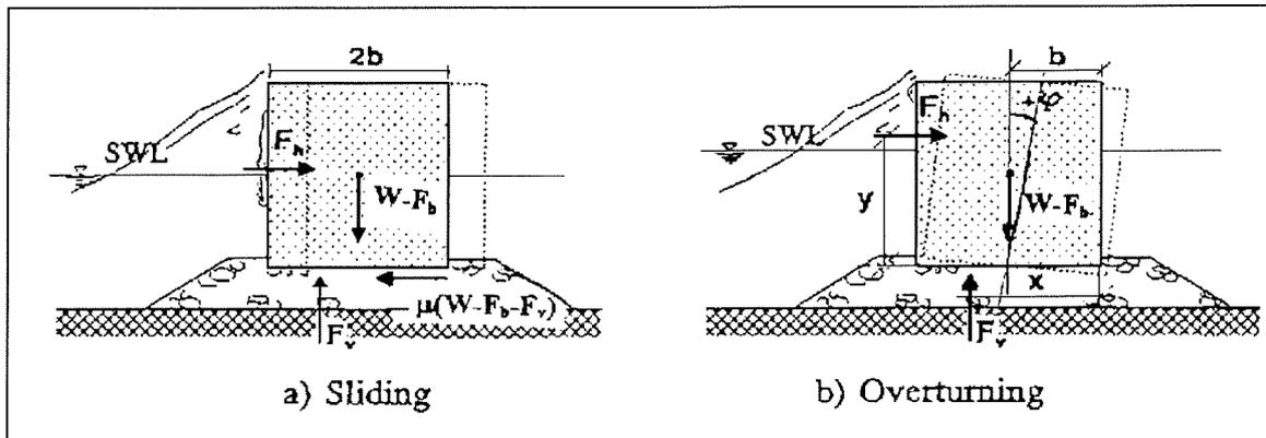
Figure 7-3 Overall failure modes [Oumeraci 1994]
