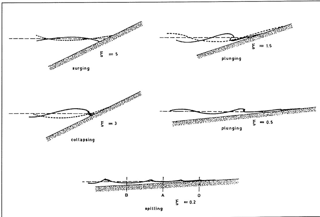
Figure 3-1 Different types of breaking wave [Battjes 1974]
