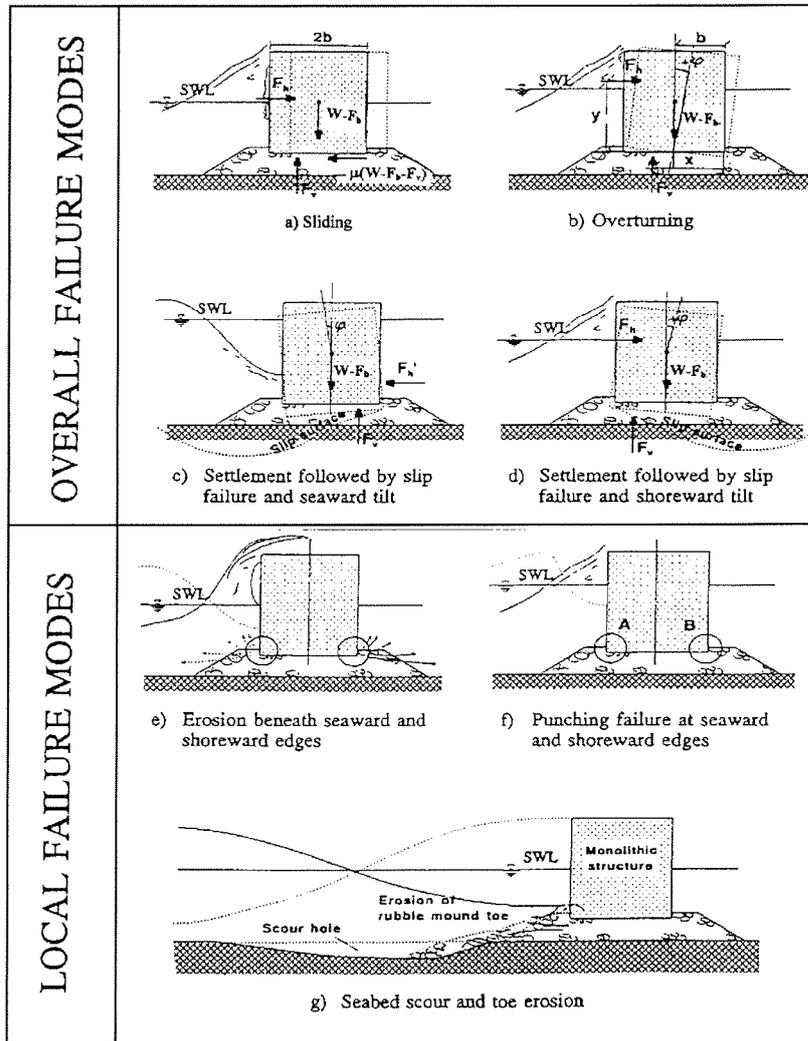
Figure 7-2 Overall and local failure modes [Oumeraci 1994]
