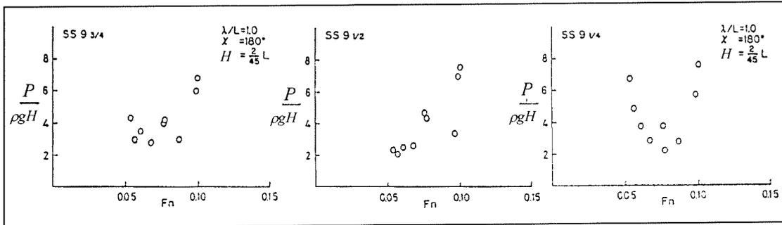
**Figure 5-4 Impact pressure vs Froude number ( $F_n$ ) [Watanabe 1987]**
