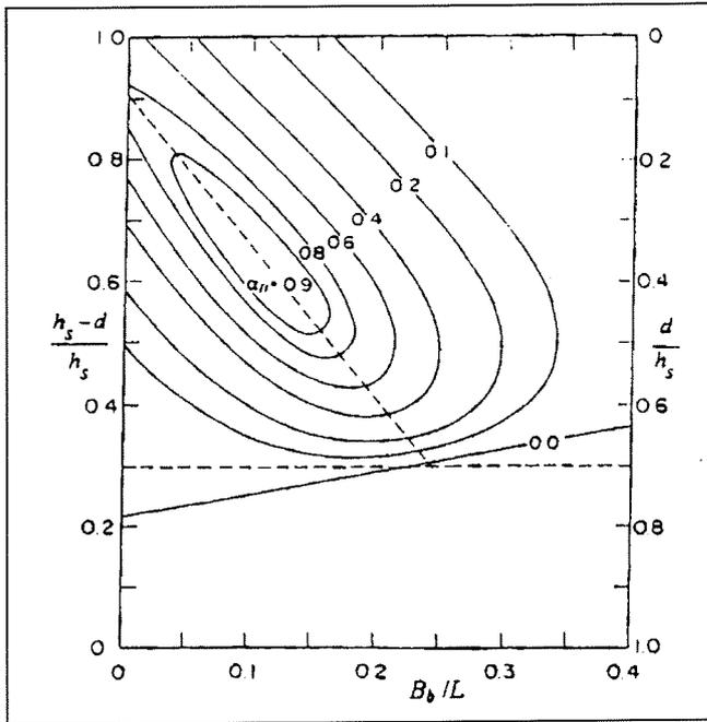
**Figure 4-9 Calculation diagram of impulsive pressure coefficient [Takahashi]**
