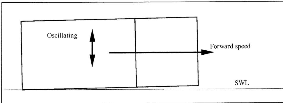
Figure 5-15 Side view of wedge entering the water
