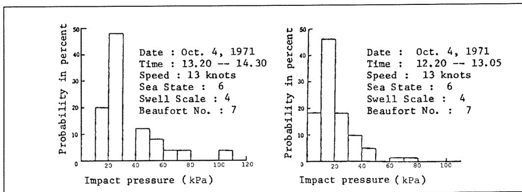
Figure 5-9 Probability of impact pressure, full scale measurements [SR 124 rep.140, 1971]
