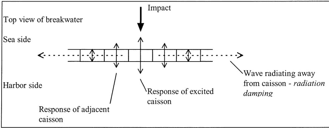
**Figure 6-2 Geometrical damping - Interlocking of caissons**
