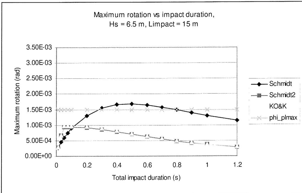
Figure 9-6 Rotation vs impact duration,  $L_{\text{impact}} = 15 \text{ m}$
