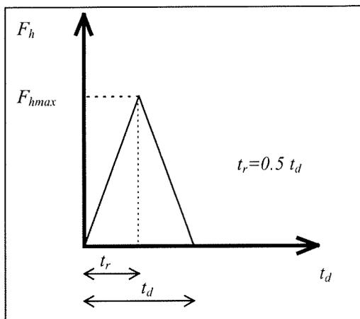
**Figure 4-7 Triangular force-time diagram**
