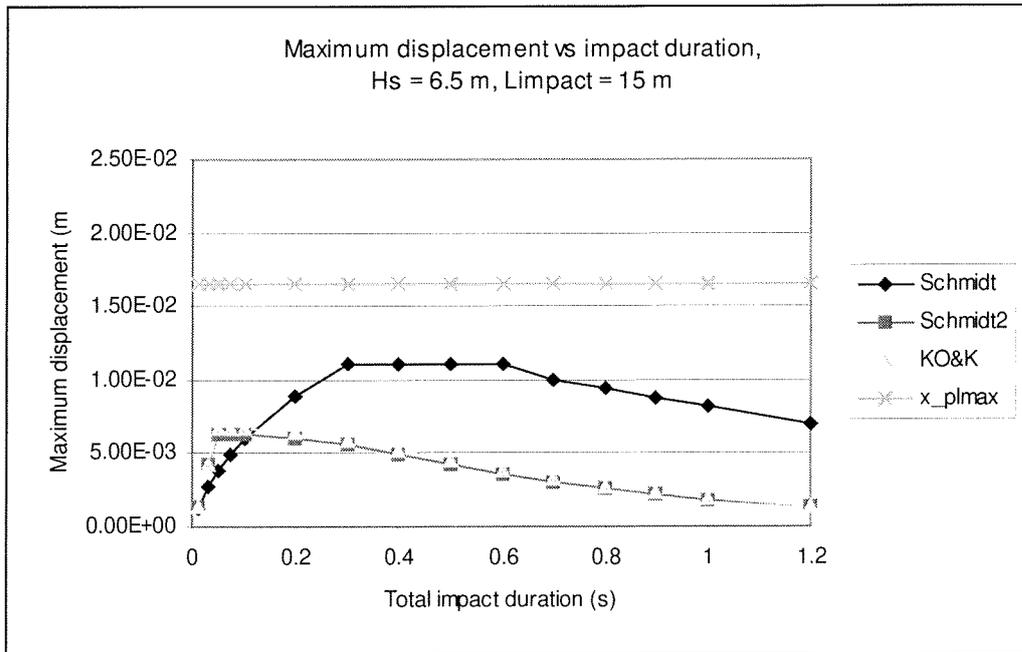
**Figure 10-2 Displacement vs impact duration,  $L_{\text{impact}} = 15$  m**
