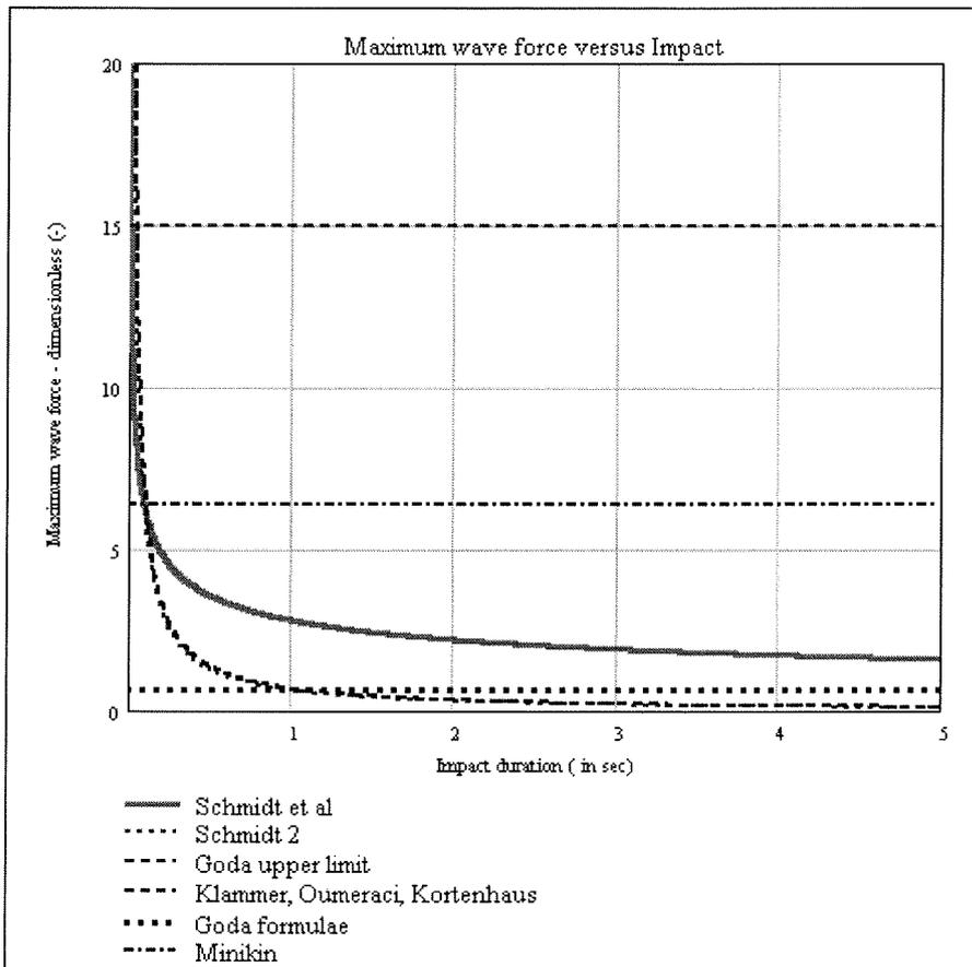
**Figure 4-13 Comparison wave impact formulae (linear scale)**
