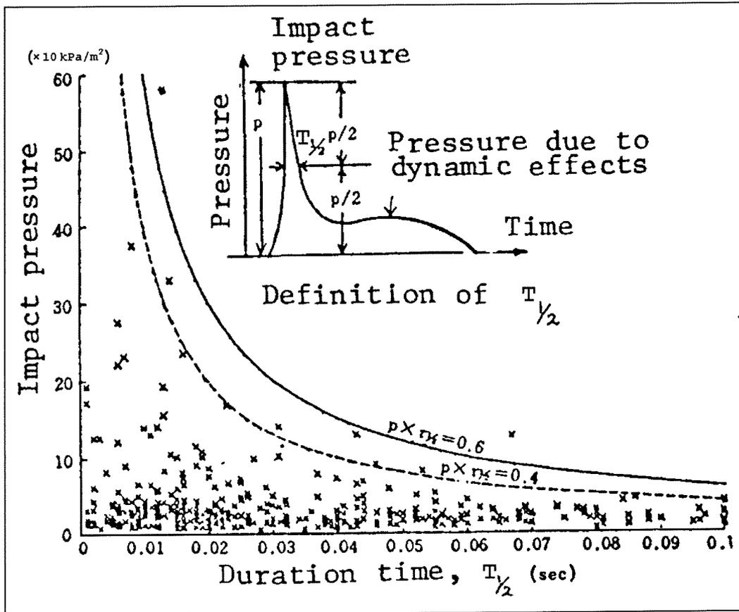
Figure 5-8 Impact pressure vs impact duration, full scale [SR 124 rep. 140, 1971]
