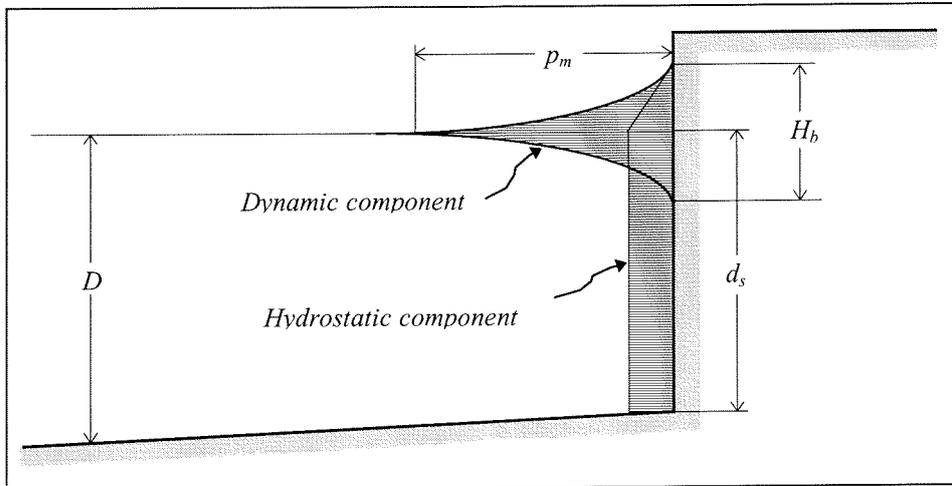
**Figure 4-8 Pressure distribution according to Minikin**
