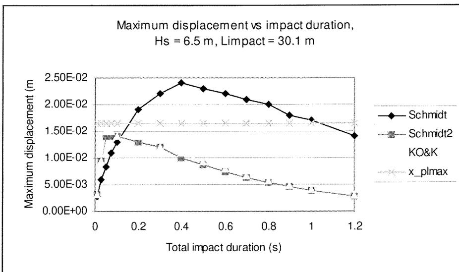
Figure 9-3 Displacement vs impact duration,  $L_{impact} = 30m$
