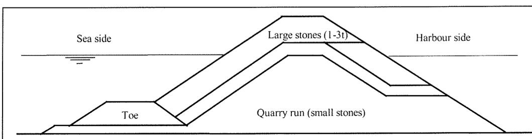
Figure 1-1 Cross-section of a rubble mound breakwater
