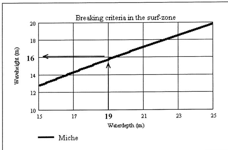
**Figure 4-11 Wave breaking in the surf zone**
