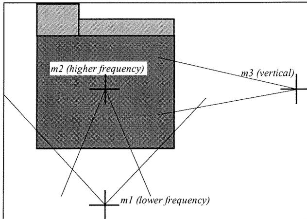
Figure 8-2 Scheme of modes of oscillations
