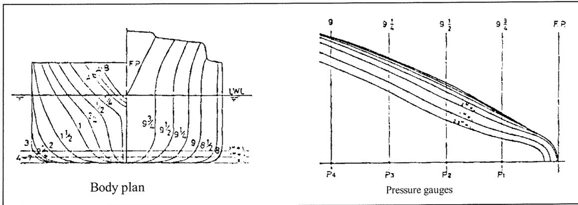
**Figure 5-2 Body plan, waterline and location pressure gauges of model [Watanabe 1987]**
