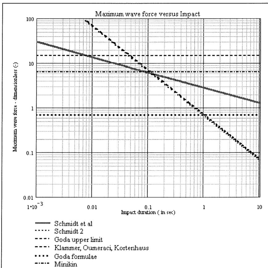
Figure 4-12 Comparison wave impact formulae (double logarithmic scale)
