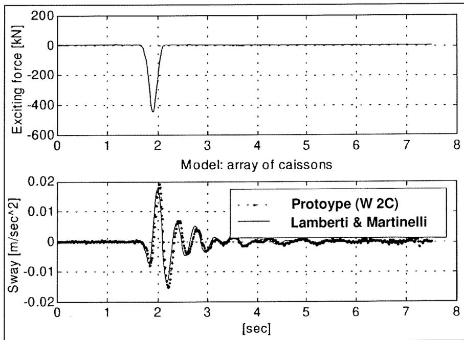
**Figure 8-3 Tugboat excitation Genoa Voltri breakwater [Lamberti & Martinelli (1998)]**
