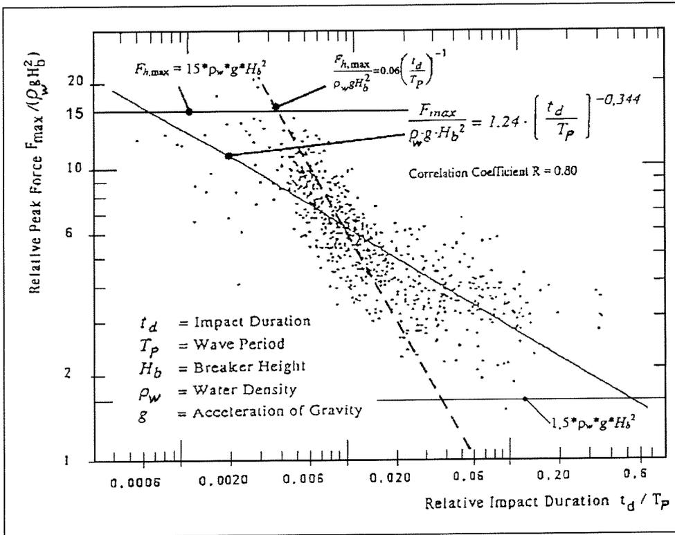
Figure 4-10 Maximum impact force vs. impact duration [Schmidt et al 1992]
