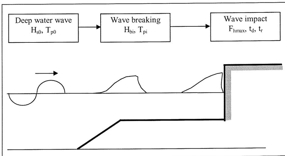
**Figure 4-4 Scheme of impulsive wave load**
