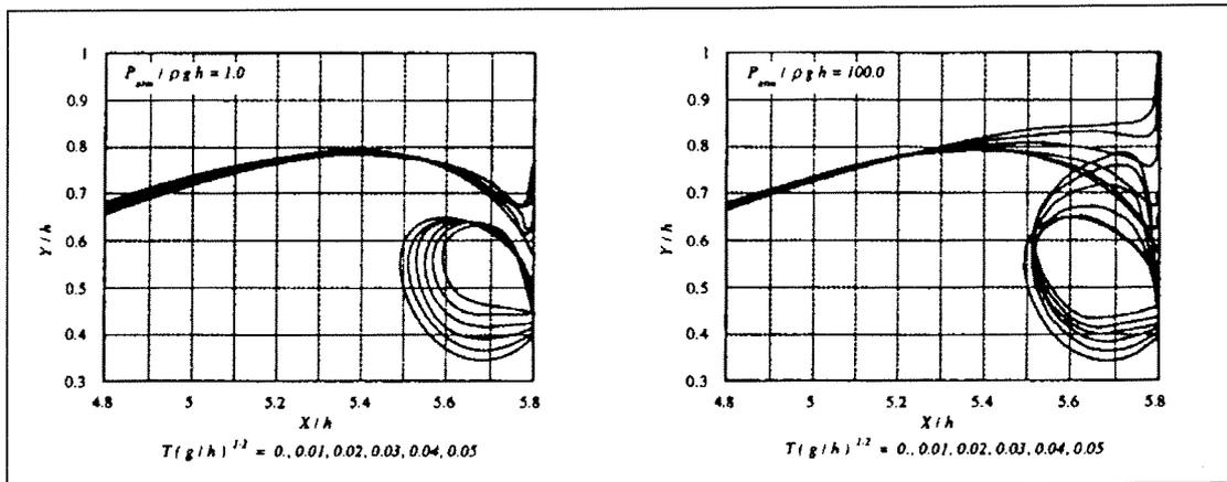
**Figure 5-16 Free surface profiles of simulated plunging wave impact [Tanizawa & Yue]**
