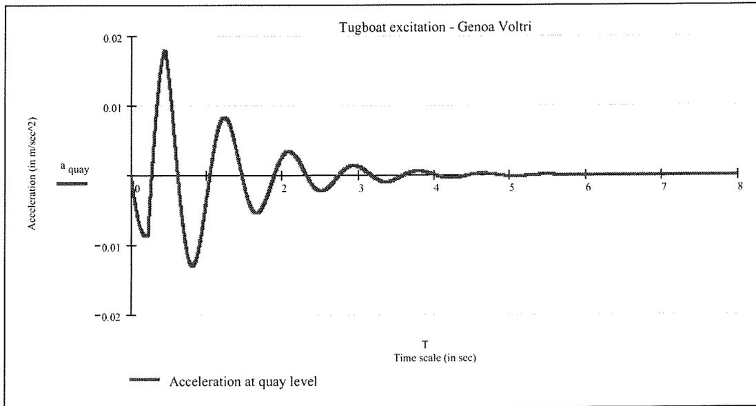
**Figure 8-4 Calculation tugboat excitation Genoa Voltri breakwater**
