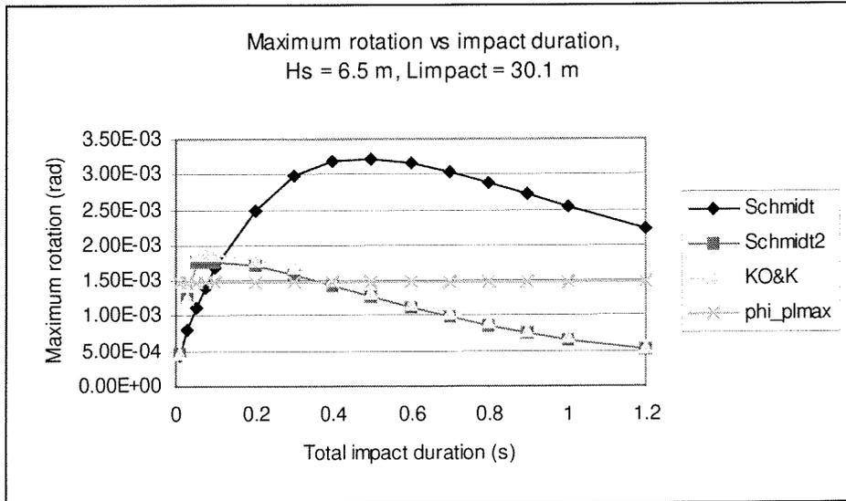
Figure 9-4 Rotation vs impact duration,  $L_{impact} = 30m$
