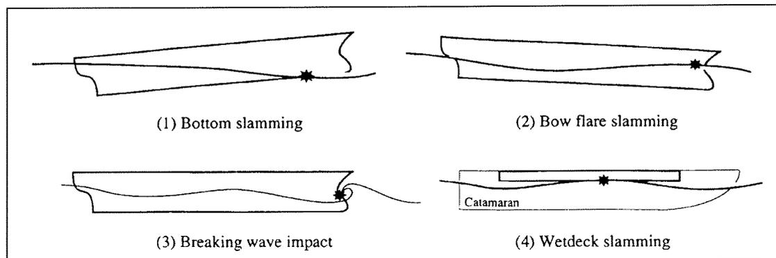
**Figure 5-1** Types of slamming impact of a ship
