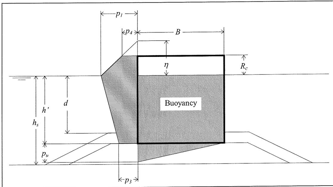
**Figure 4-3 Model of non-breaking and breaking waves by Goda**
