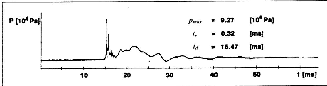
Figure 5-20 Pressure history on wall with air entrapment [Schulz 1992]
