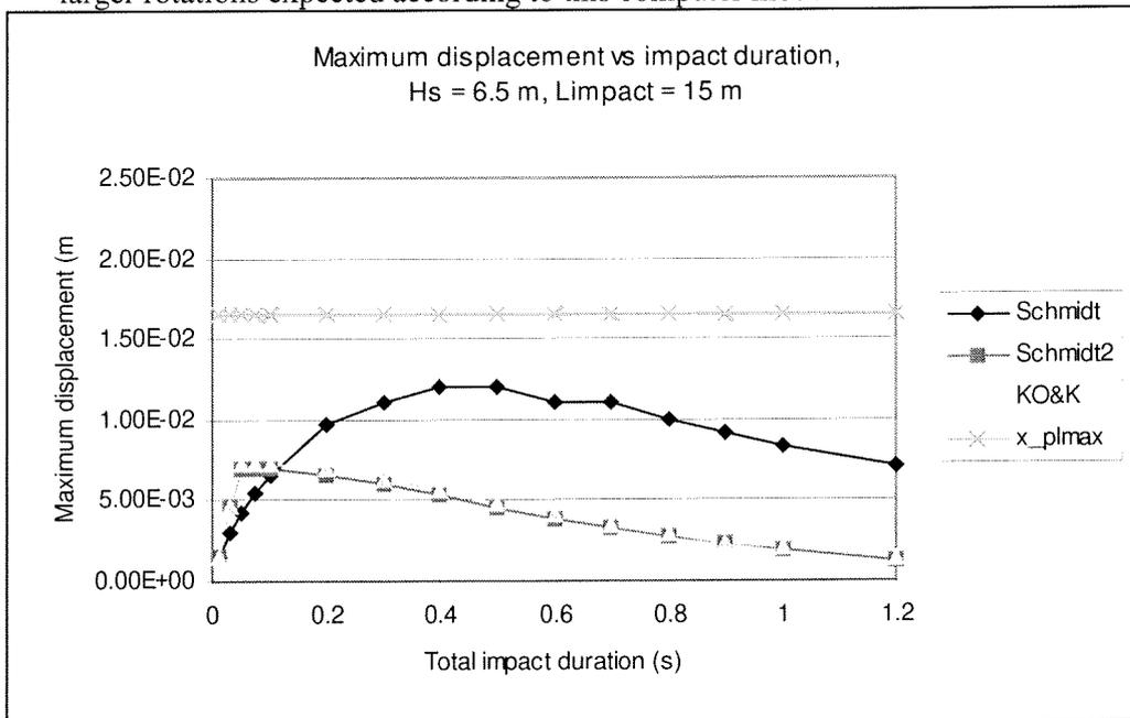
Figure 9-5 Displacement vs impact duration,  $L_{impact} = 15 m$
