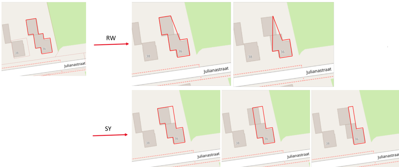
Figure 5.4.: An example of a situation where Reumann-Witkam results in a 'pointy' structure, while the Samsonov-Yakimova algorithm preserves the initial structure
