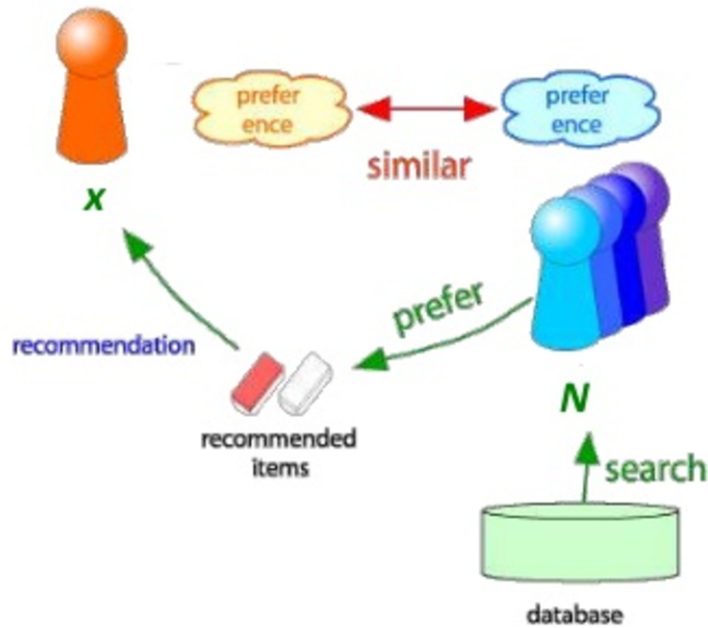
Figure 2.3: Work-flow of CF Recommendation[46]. In this work-flow, the X users' profile is created based on expressed preferences. Then we find a set of N users whose preferences are similar to user X's preferences. Then estimate user X's ratings based on ratings of users in N. Highest rated items are recommended to user X.
