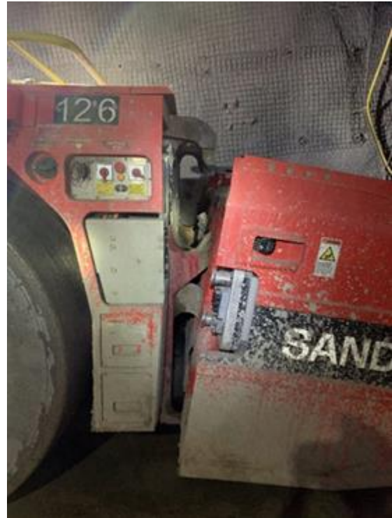
Figure 11: Images of the Autoswap process and its complications when vehicle and battery are not aligned (sent from New Afton)
