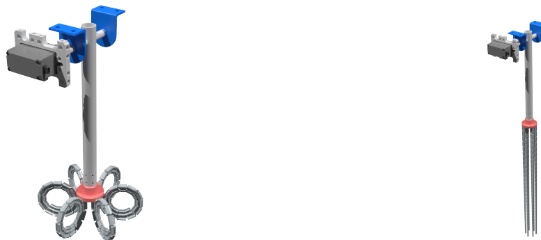
Figure 8.4: Final renders of grabber subsystem, (a) when tentacles are fully curled up, (b) when tentacles are fully extended.
