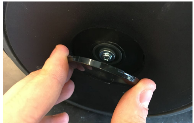
Fig. 151, Removal of the semi-transparent screw cover in the Samsung SC8835
