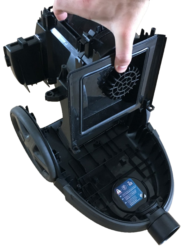
Fig. 142, 3 steps disassembly of the motor assy. Extraction of the motor assy in a Philips Power Pro Active.
