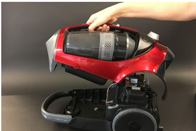
Fig. 82, Upper plastic clump disassembly of the Samsung SC8835
