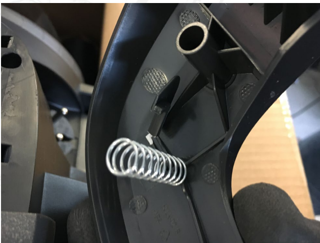
Fig. 78, Broken hidden snap fit after an official repairer tried to disassemble one of the upper buttons
