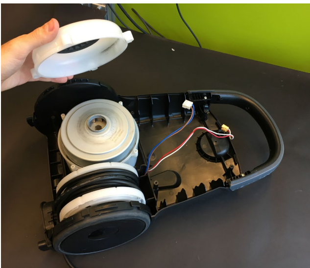
Fig. 146, One step vertical disassembly of the motor housing lid in a Samsung SC8835
