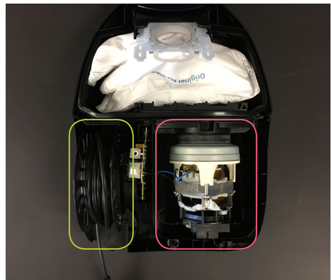
Fig. 136. Independent disassembly of motor and cord-winder in Siemens SyncroPower
