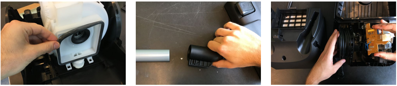
Fig. 18, Examples of Friction fits by hand (force type 1, 2 and 3)
