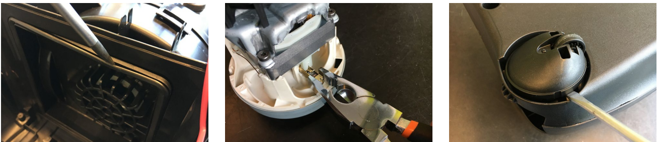
Fig. 19, Examples of Friction fits using a spudger (force type 1, 2 and 3)
