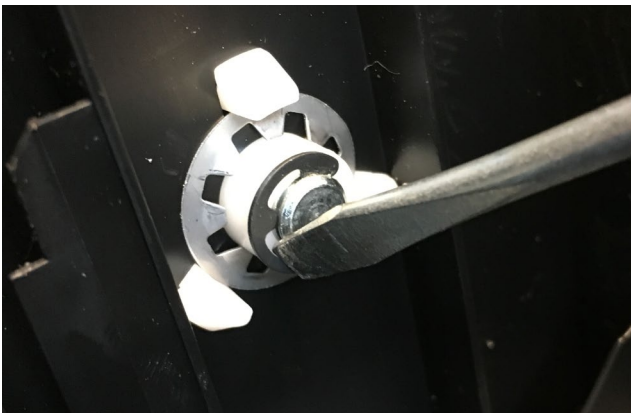
Fig. 148, Bearing wheel fastening system in the Philips Power Pro Ultimate
