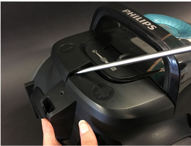
Fig. 76, Top buttons disassembly, using a spudger (High force intensity hidden snap fit connectors)
