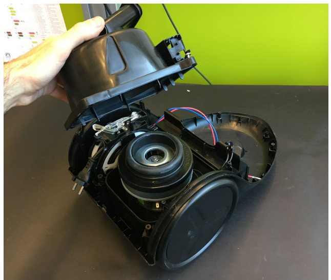
Fig. 147, One step vertical disassembly of the motor housing lid in a Rowenta X-Trem
