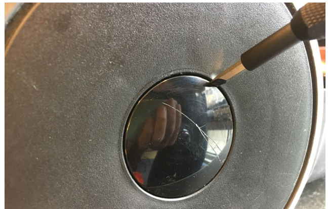
Fig. 150, Semi-transparent cover, hiding the wheel screw in the Samsung SC8835
