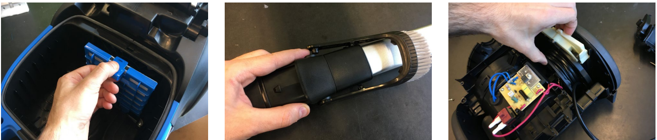
Fig. 20, Examples of Snap fits by hand (force type 1, 2 and 3)
