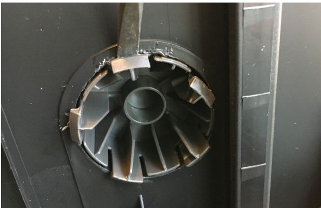
Fig. 149, Snap fits wheel fastening system in the Philips Power Pro Active
