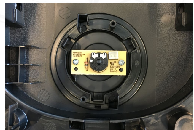
Fig. 101, Power knob assembled from the inside towards the outside in a FC85XX.
