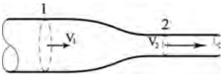
Figure 4.6 ..... Venturi effect: a decrease in the cross-sectional area (from 1 to 2) results in an increase of the fluid average velocity (from v_1 to v_2 ). .....
