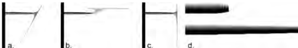
Figure 7.24 ..... The shading sheets inclination and their support elongation. (a.-c.) showing different inclinations of the sheet connected to the support member by an elastic membrane. (d) the support tubular member elongation. .....
