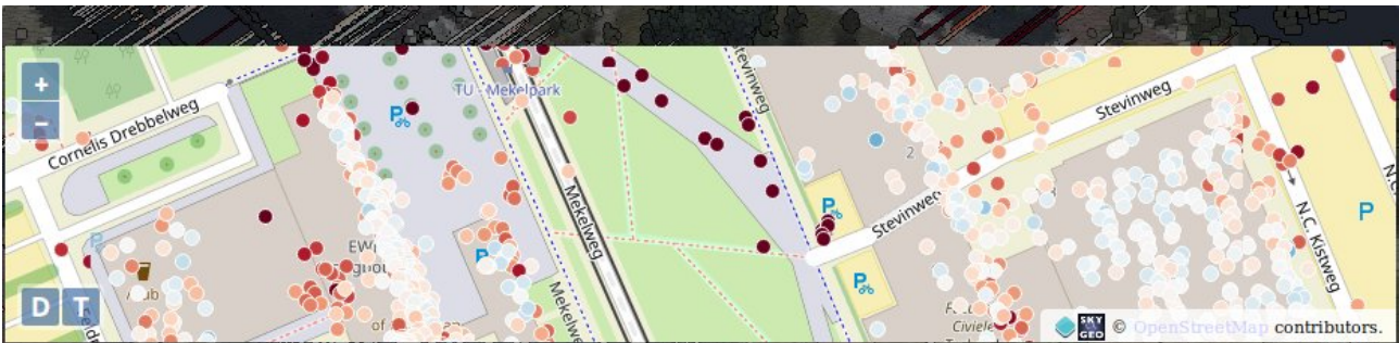
Figure 27: Map, as shown in the viewer. Scatterers are marked with dots and coloured according to their deformation velocity.
