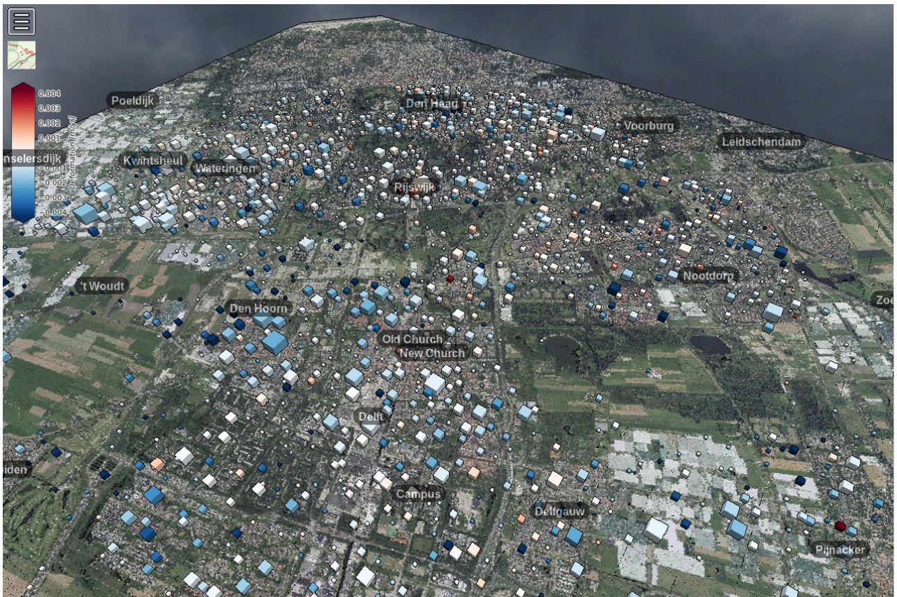
Figure 25: Clustering of 1 million persistent scatterers in 1500 clusters. Size of the cluster related to the points in the cluster, color indicates (average) deformation speed of the cluster. (Vertical scaling factor: 5000.)
