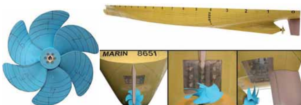
Figure 7.4: Model propeller (left) and experimental set-up (right) for container vessel #3.
