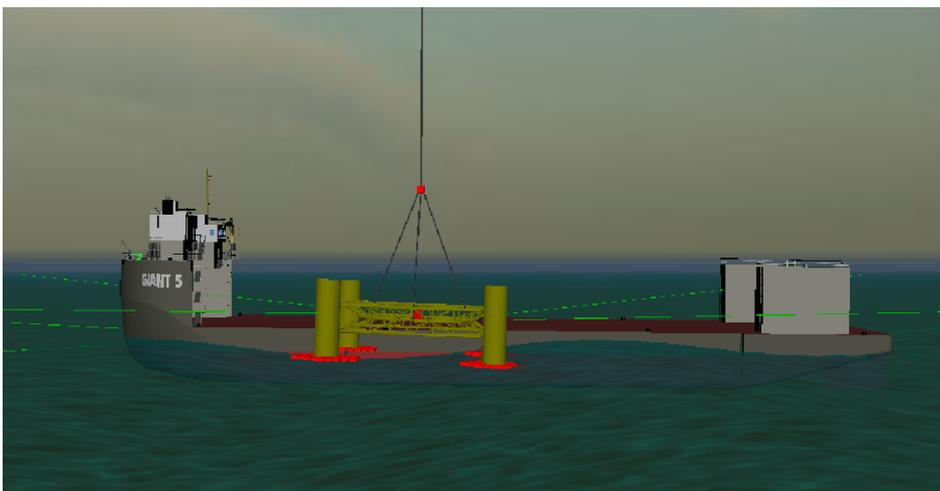
*Figure 3.24: OrcaFlex model side view*
