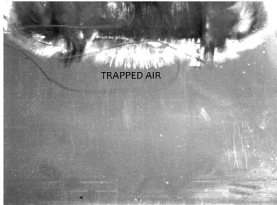
*Figure 2.3: Frame taken by high speed camera after initial water entry capturing trapped air, F.J. Huera-Huarte [8]*
