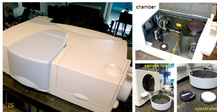
Figure 3. 3: PerkinElmer® Lambda 1050 spectrophotometer with Integrating sphere setup [34].
