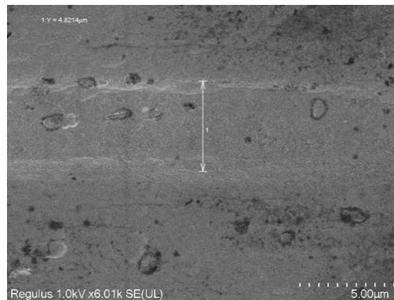
Figure 4. 45: SEM image of baseline carrier foil with TCO
