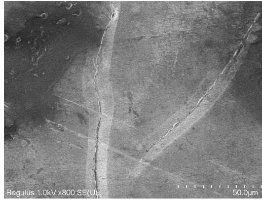
Figure 4. 47: SEM image of TCO + Carrier foil with cracks
